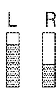
LEFT AND RIGHT SOUND IMAGES WHEN ELEVATION IS 45 DEGREES
