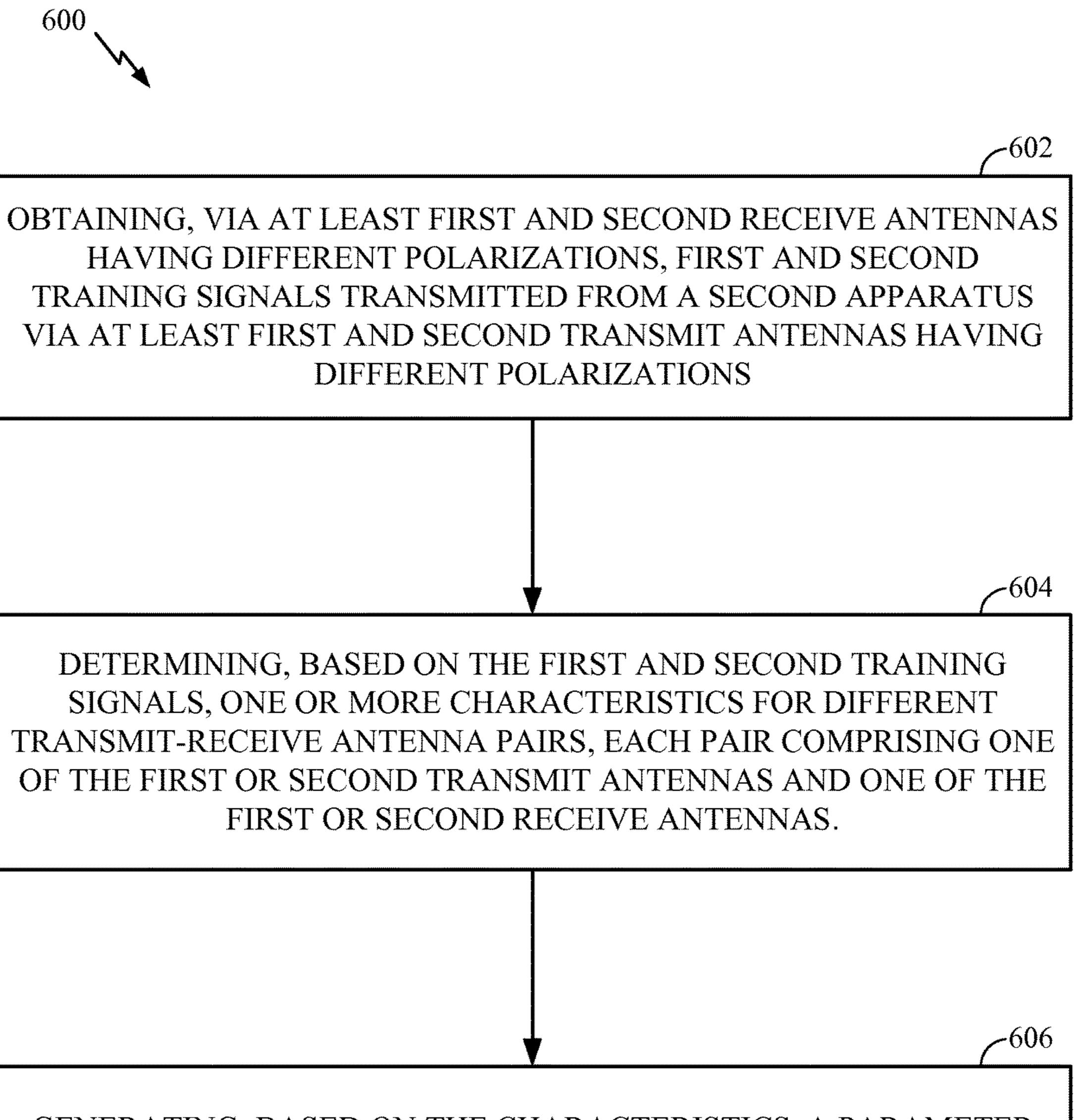
GENERATING, BASED ON THE CHARACTERISTICS, A PARAMETER INDICATIVE OF WHETHER A LINK PATH BETWEEN THE FIRST AND SECOND APPARATUS IS LINE OF SIGHT (LOS).
