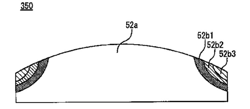
having a higher content rate of heavy rare earth element than that of the first magnetic powder, at a predetermined position in the cavity.
