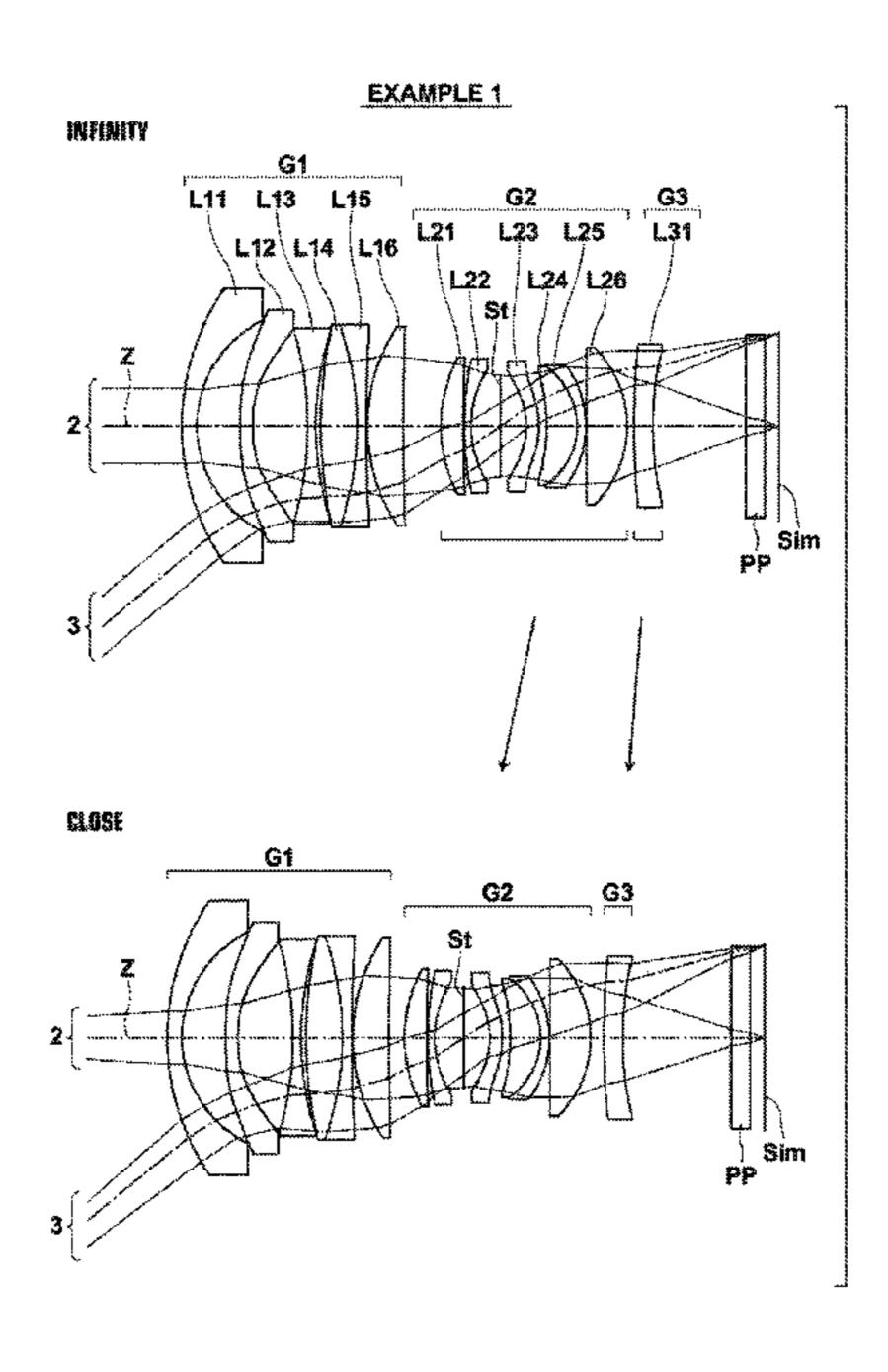
distance between the second lens group and the third lens group changes while the first lens group is fixed. The first lens group includes, consecutively in order from the most object-side, a negative first lens and a negative second lens.
