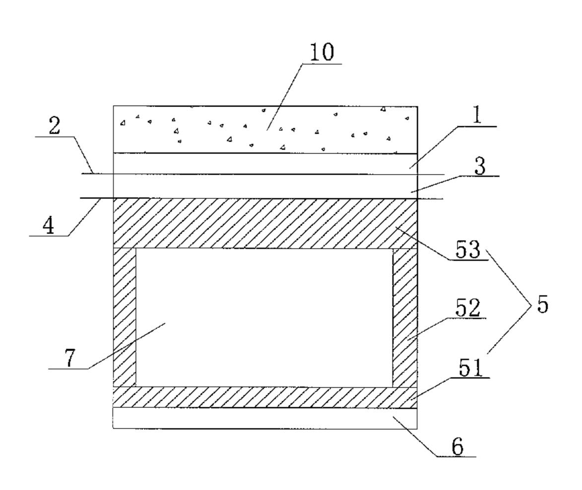
layer (7) varies from  $1 \times 10^{-5}$  to  $1 \times 10^{-3}$ . A method of manufacturing the MSW landfill barrier system capable of prolonging breakthrough time of leachate is also provided.
