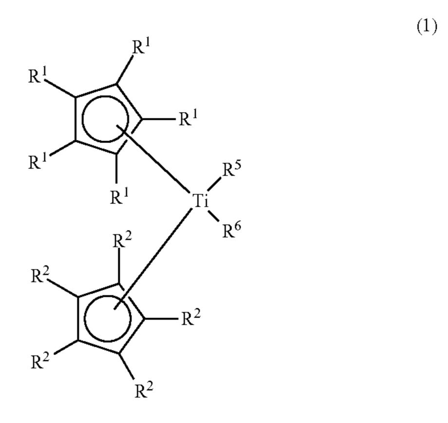
(wherein R<sup>5</sup> and R<sup>6</sup> are any group selected from hydrogen, a hydrocarbon group having 1 to 12 carbon atoms, an aryloxy group, an alkoxy group, a halogen group, and a carbonyl group. R<sup>1</sup> and R<sup>2</sup> are any group selected from the group consisting of hydrogen and a hydrocarbon group having 1 to 12 carbon atoms, and R<sup>1</sup> and R<sup>2</sup> are not all hydrogen atoms or all a hydrocarbon group having 1 to 12 carbon atoms),
