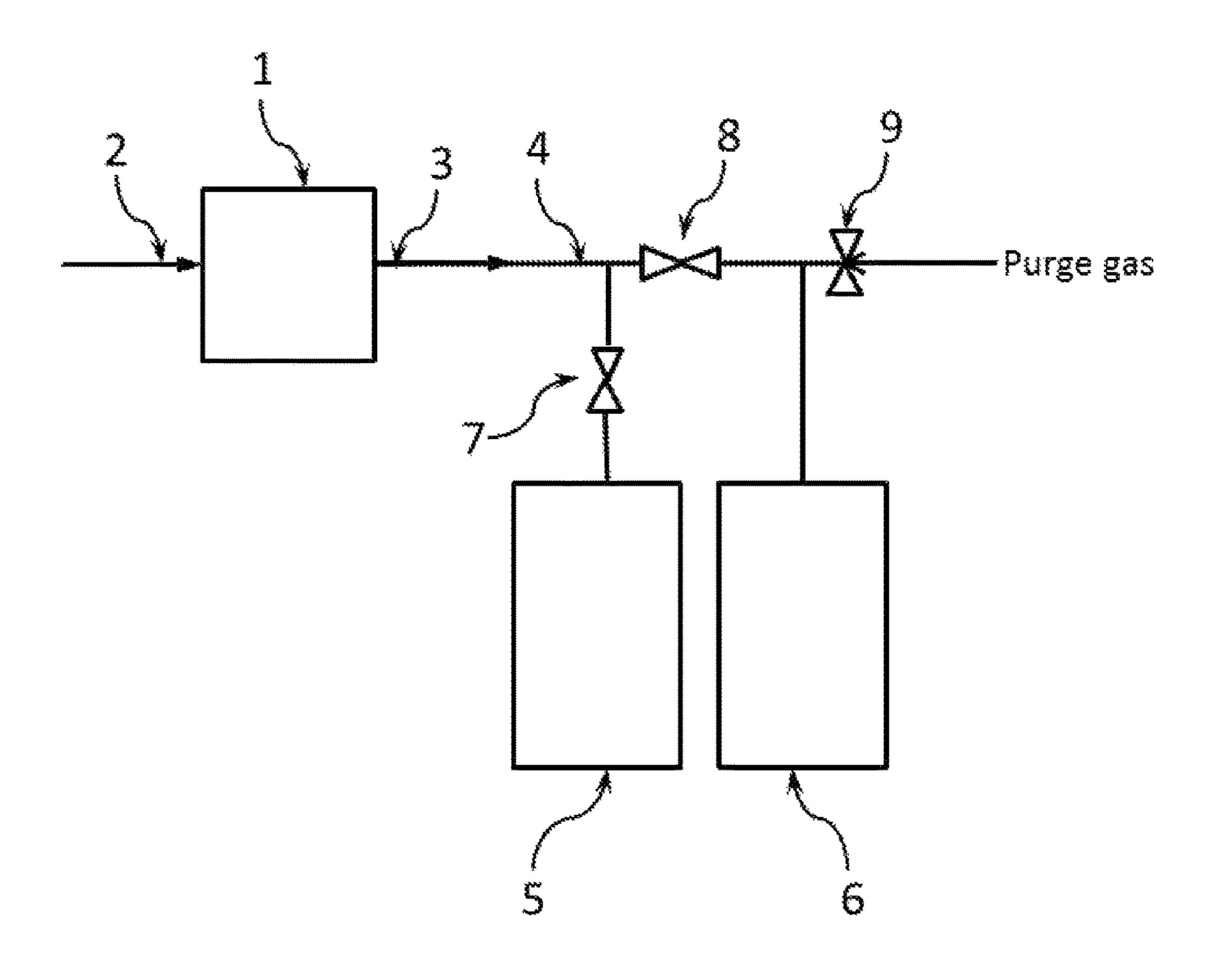
FIGURE 3: Withdrawal System having Two Purge Lines
