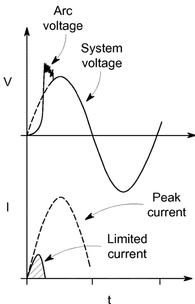
Conventional medium voltage circuit breakers are 3 to 5 cycles or 6 to 10 loops - this current limiting circuit breaker is interrupting in a fraction of a loop
