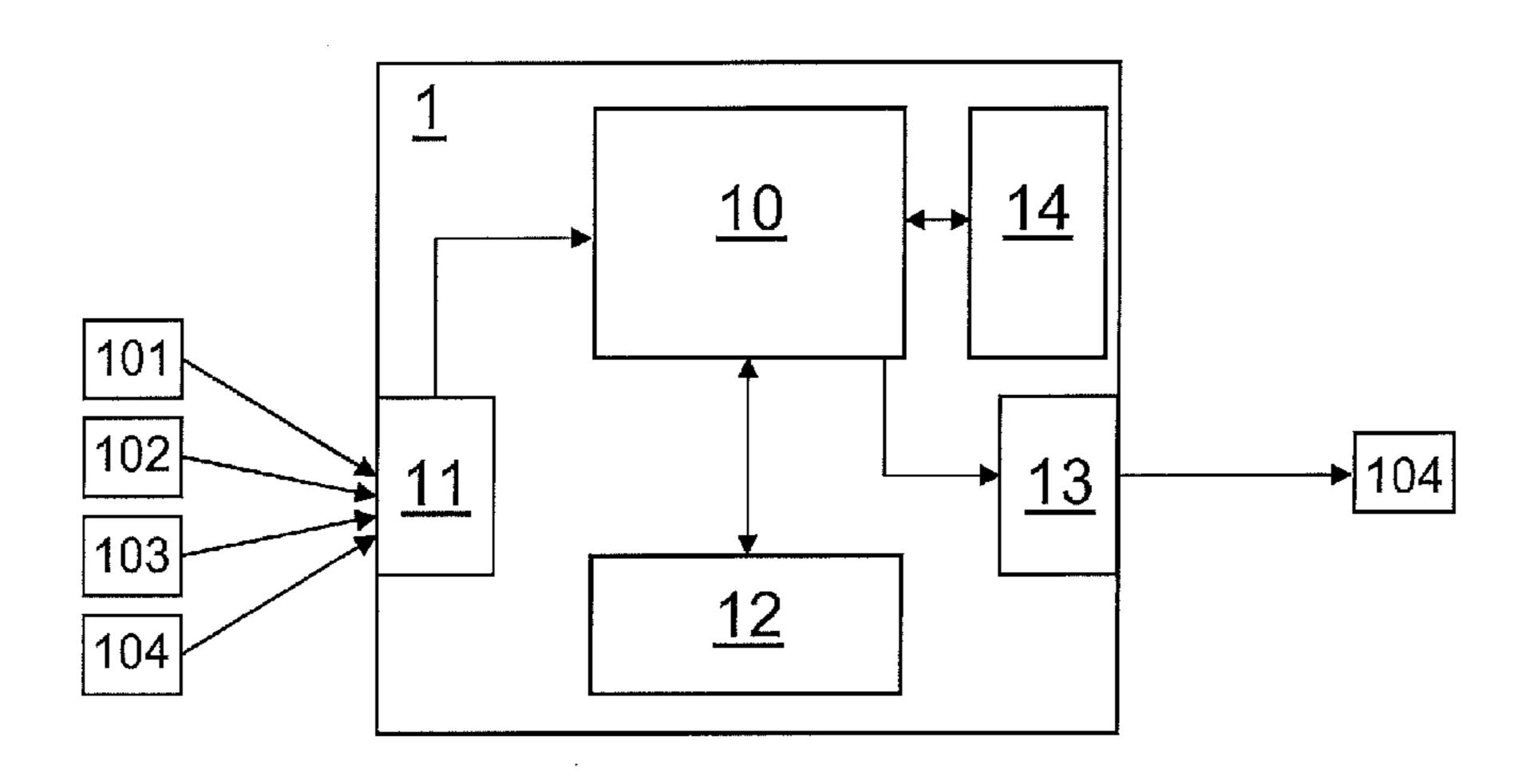
input variable ascertained during operation, at least one output variable for a control system of functions of the vehicle. The control device performs the calculation of the output variables using a Bayesian regression of training values ascertained, before operation, for the output variable and the input variable.
