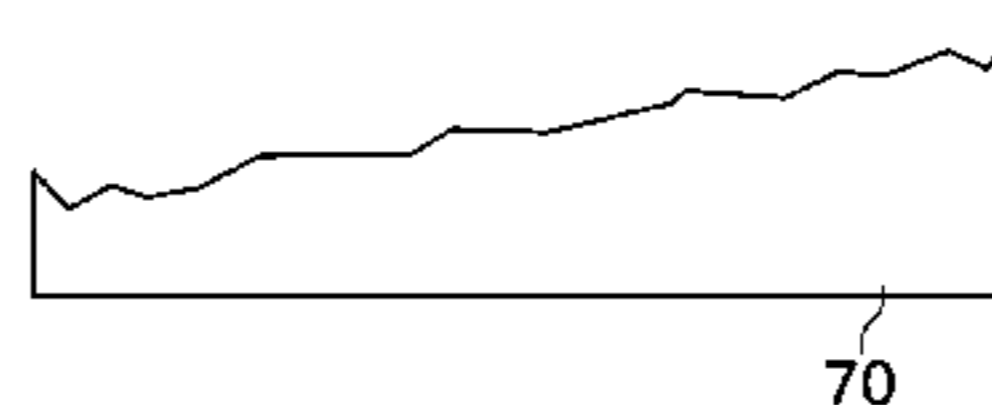
(b) SiC substrate surface after vapor-etching planarization
