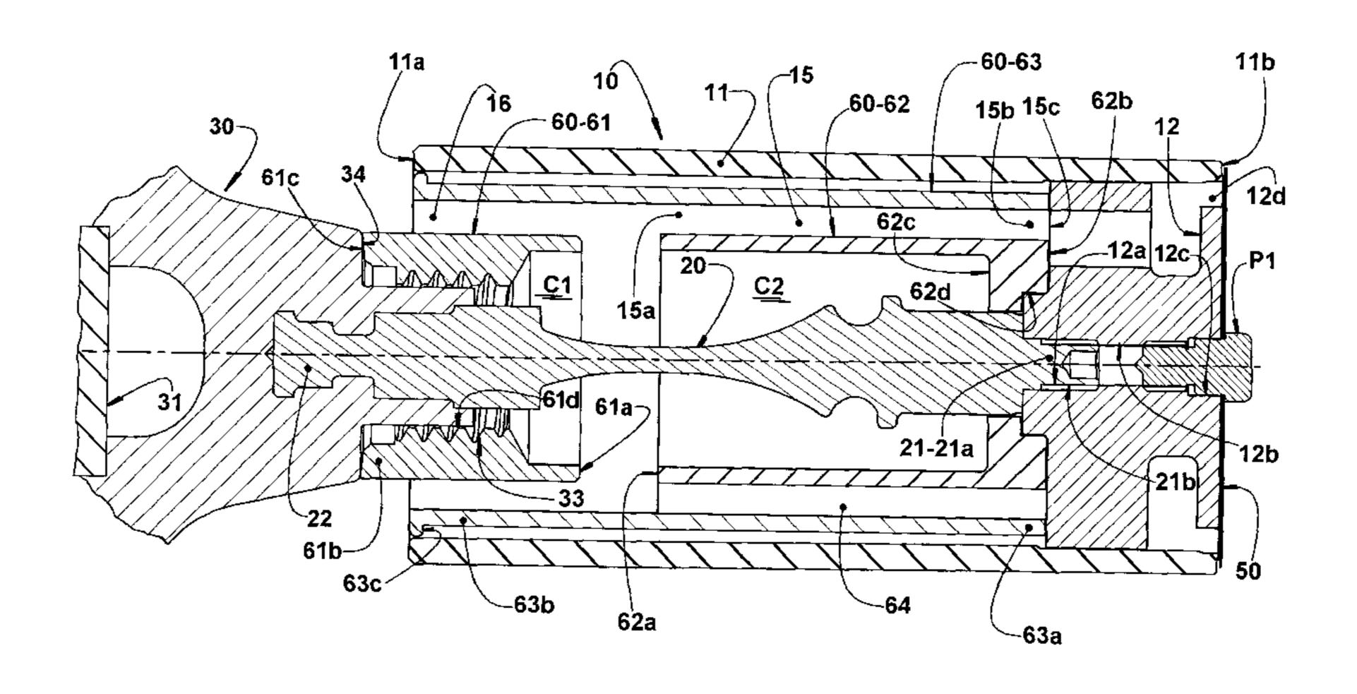
chambers (C1, C2), and communicating the open rear end (11a) of the skirt (11) with the suction valve (50).
