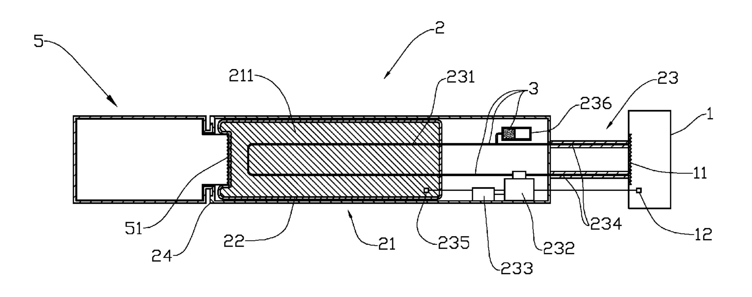
cooling circuit (23) being thermally coupled to a downhole tool (1) being in the need of cooling during downhole operations.
