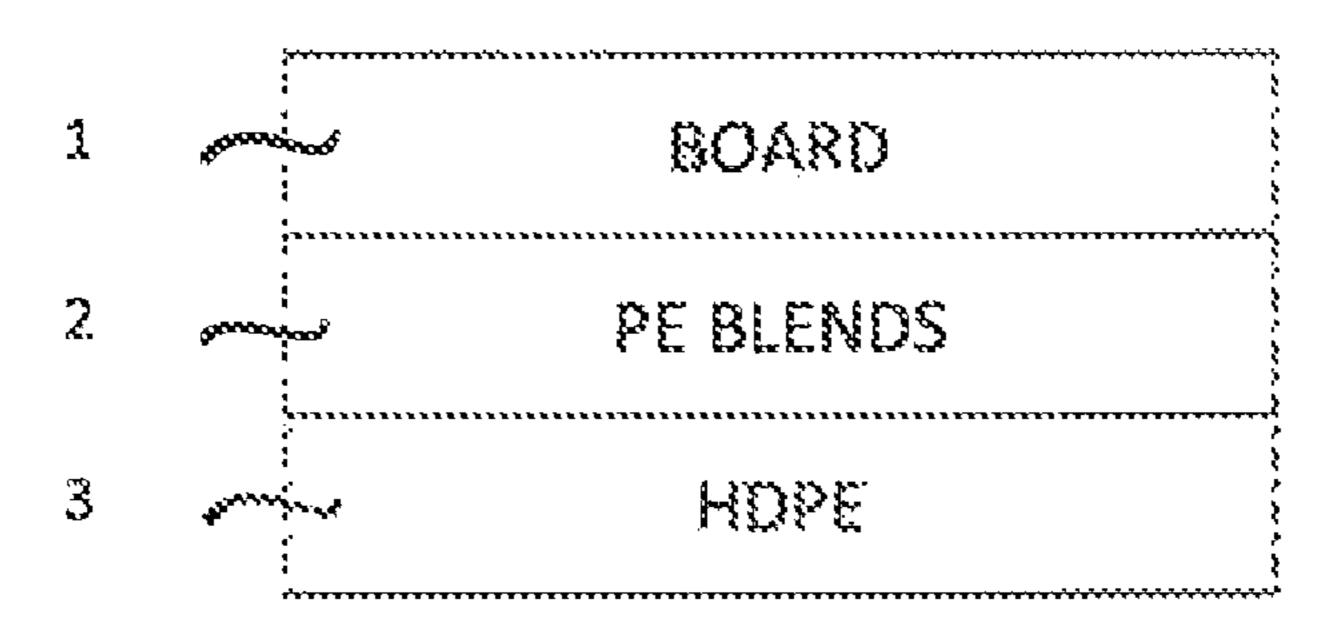
To maximize renewability of the materials HDPE and LLDPE as used for the structure are of biologic origin.
