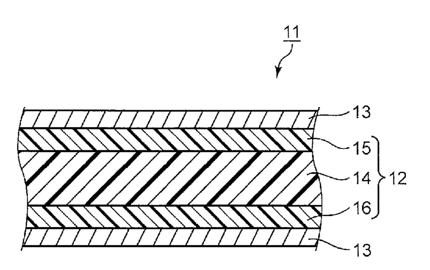
layer. A relative permittivity of the cured product of the resin composition included in the second resin layer is lower than a relative permittivity of the cured product of the resin composition included in the first resin layer.
