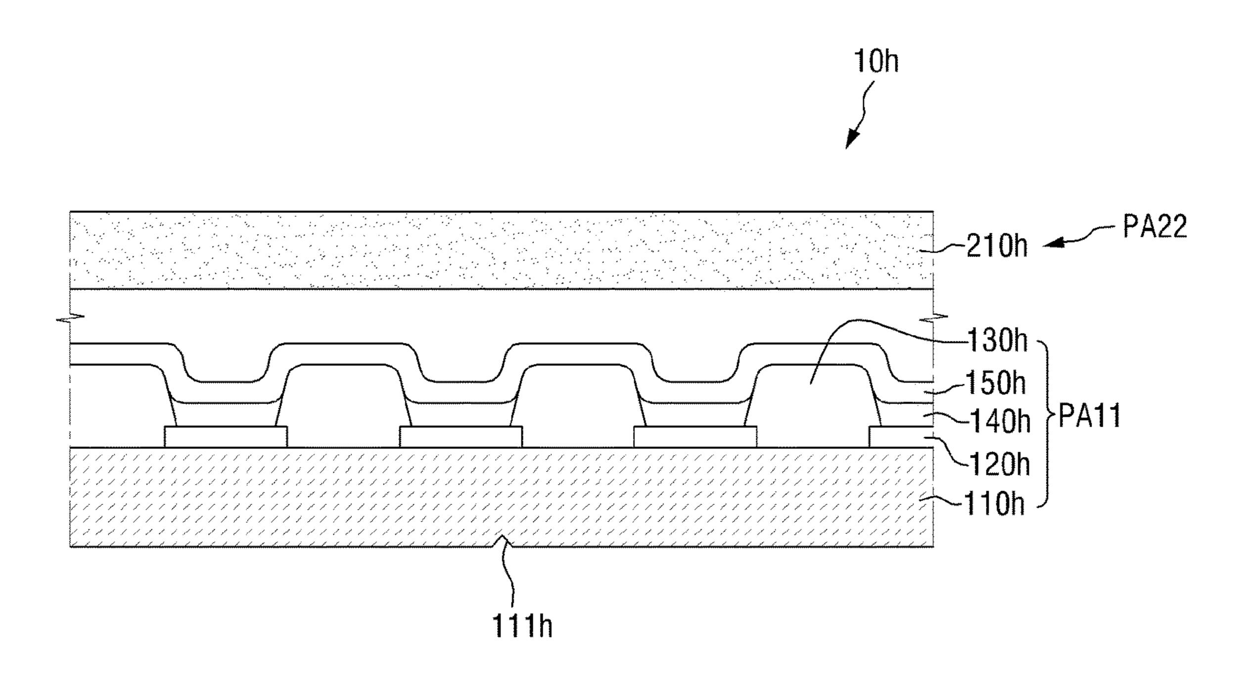
DISPLAY PANEL COMPRISING FIRST AND SECOND SUBSTRATES HAVING CRACK GUIDE GROOVES FORMED ON OUTER SURFACES OF THE FIRST AND SECOND SUBSTRATES FACING AWAY FROM EACH **OTHER**
