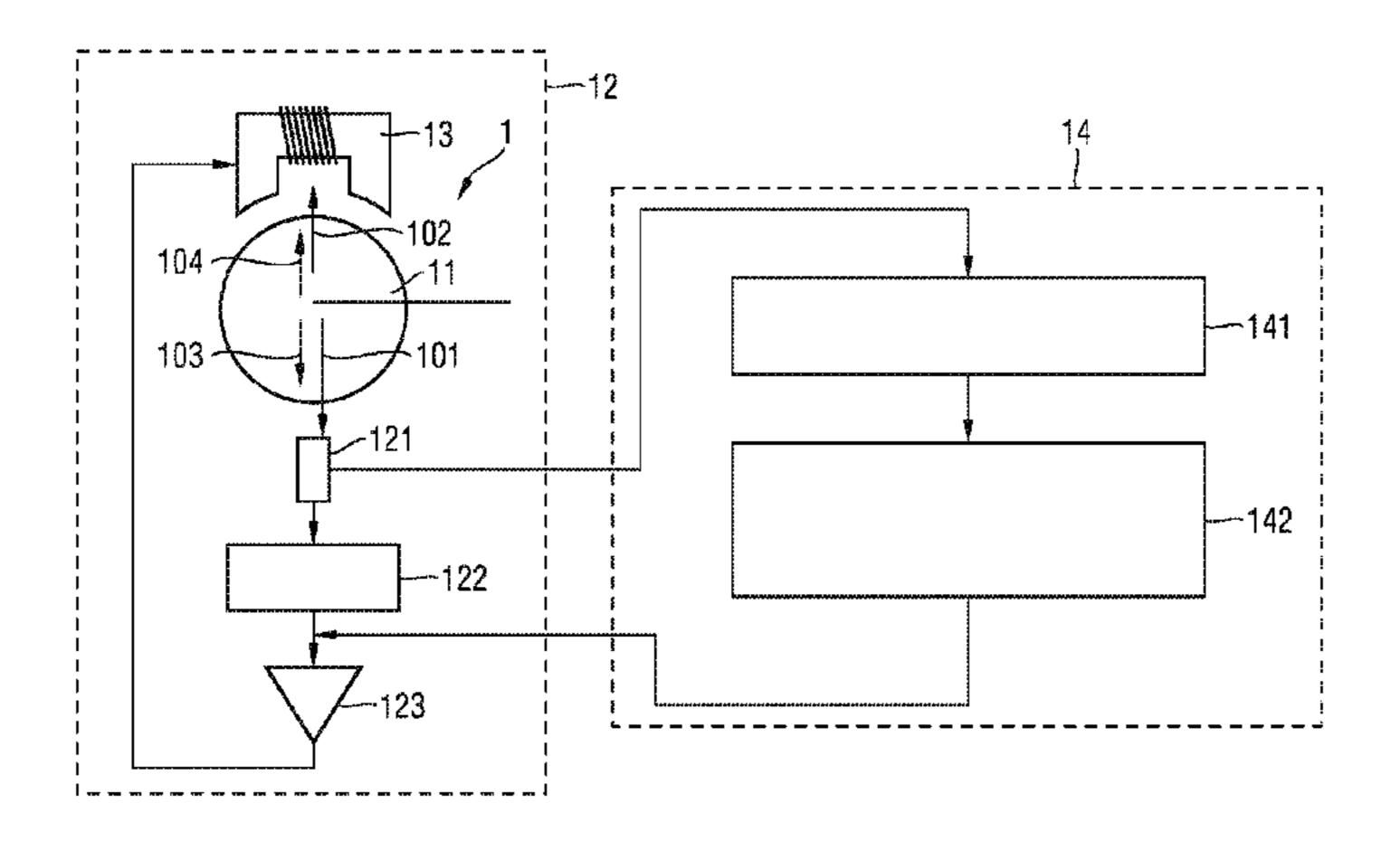
circuit of the active magnetic bearing that is decoupled from a magnetic-bearing control circuit for controlling the active magnetic bearing. The invention further relates to a corresponding active magnetic bearing.
