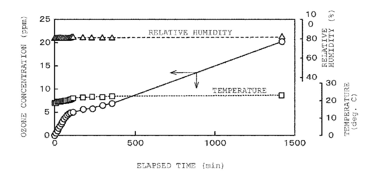
humidified ozone-containing air is preferably greater than or equal to 80%. In controlling degradation treatment on the basis of CT values, a difference between expected humidity and measured humidity is reflected in an increment of CT value to understand the progress of anticancer agent degradation properly.
