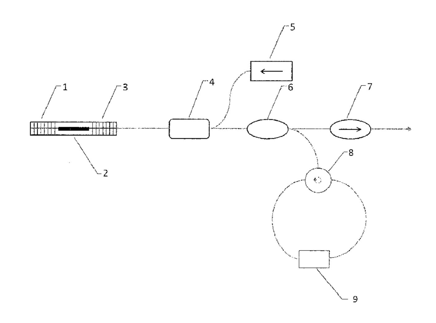
multiplexer is split by the optical coupler, a part of the laser passes through the optical circulator to enter the tunable optical filter module. A wavelength corresponding to any nominal center frequency stipulated by the ITU-T is selected by the tunable optical filter module, with a 3 dB spectral width of less than 0.1 nm, and is then injected back into the resonant cavity via the optical circulator and the optical coupler, and the resonant cavity is subjected to a self-injection locking.
