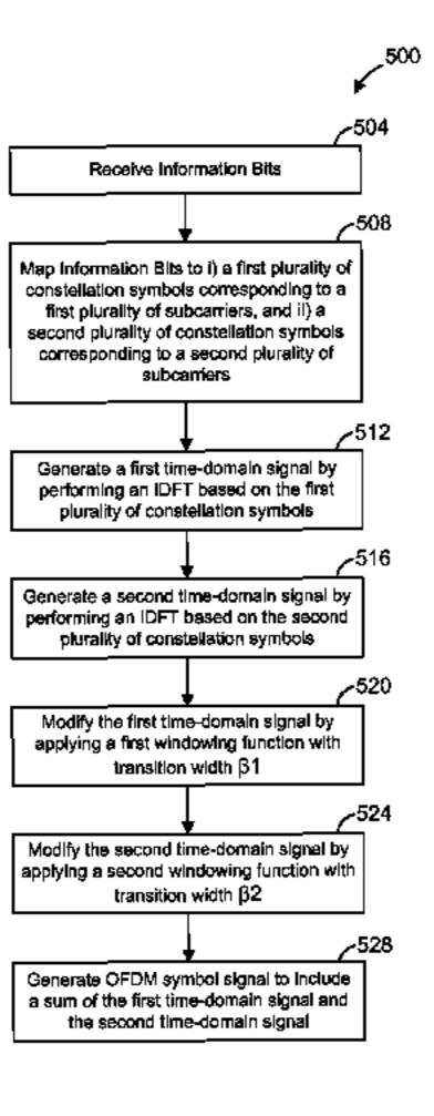
time-domain signal, the output signal corresponding to the OFDM symbol.
