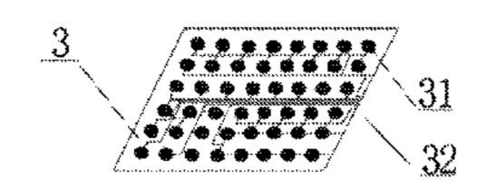
layer via glue, making the positions of the conductive dots and the holes corresponding to each other.
