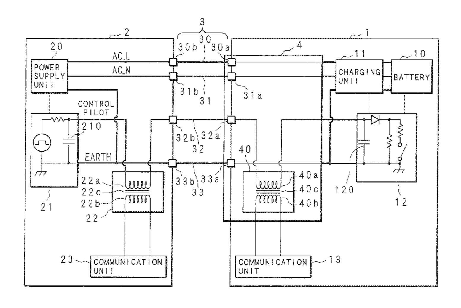
power storage device, are provided. The ratio of the winding number of a primary coil connected with at least one of the control wire and the earth wire to the winding number of a secondary coil connected with a communication unit that sends and receives a communication signal is set at 1/N (N>1) in a system which satisfies VnC>VnL or is set at N (N>1) in a system which satisfies VnC<VnL.
