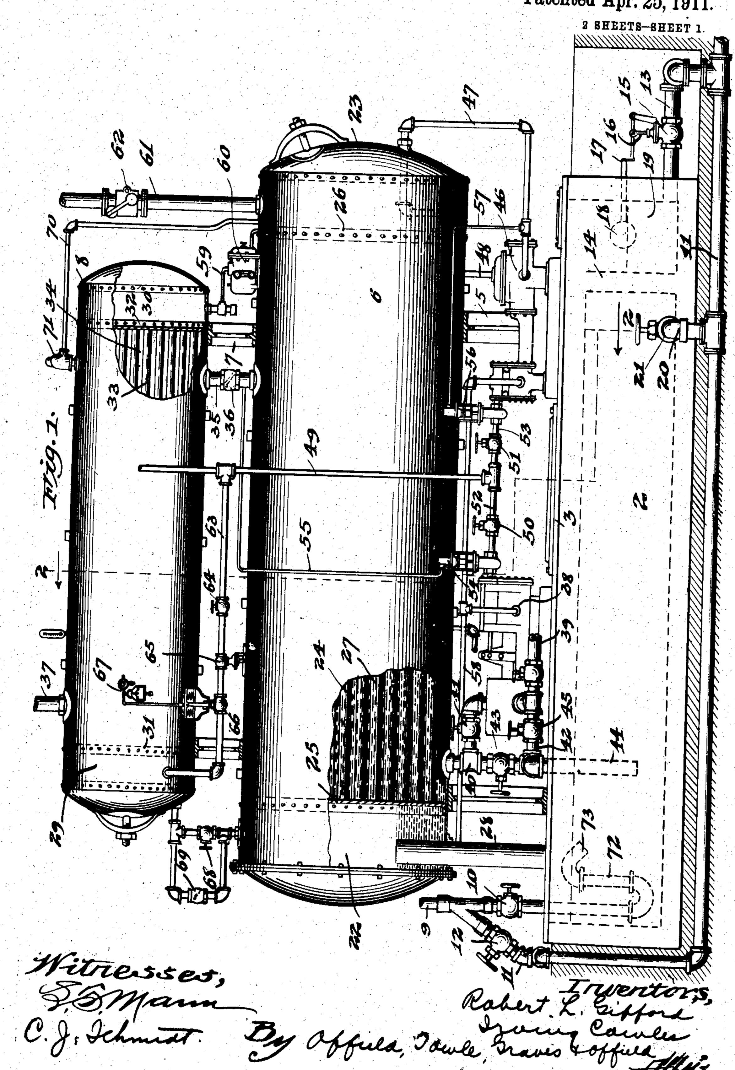
R. L. GIFFORD & I. COWLES. WASHING AND FILLING SYSTEM FOR LOCOMOTIVE BOILERS. APPLICATION FILED AUG. 27, 1909.
