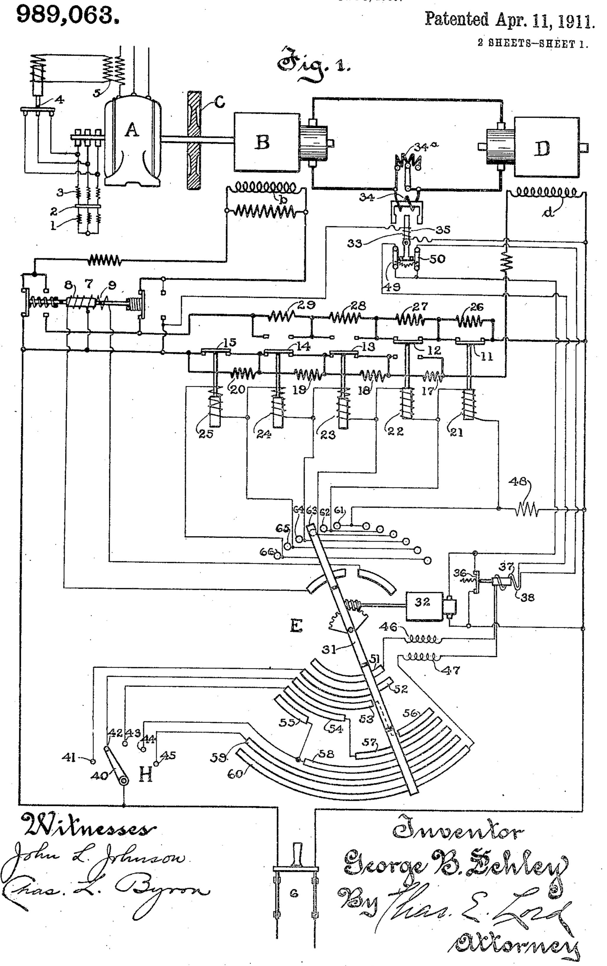
G. B. SCHLEY. SYSTEM OF MOTOR CONTROL. APPLICATION FILED JULY 8, 1909.
