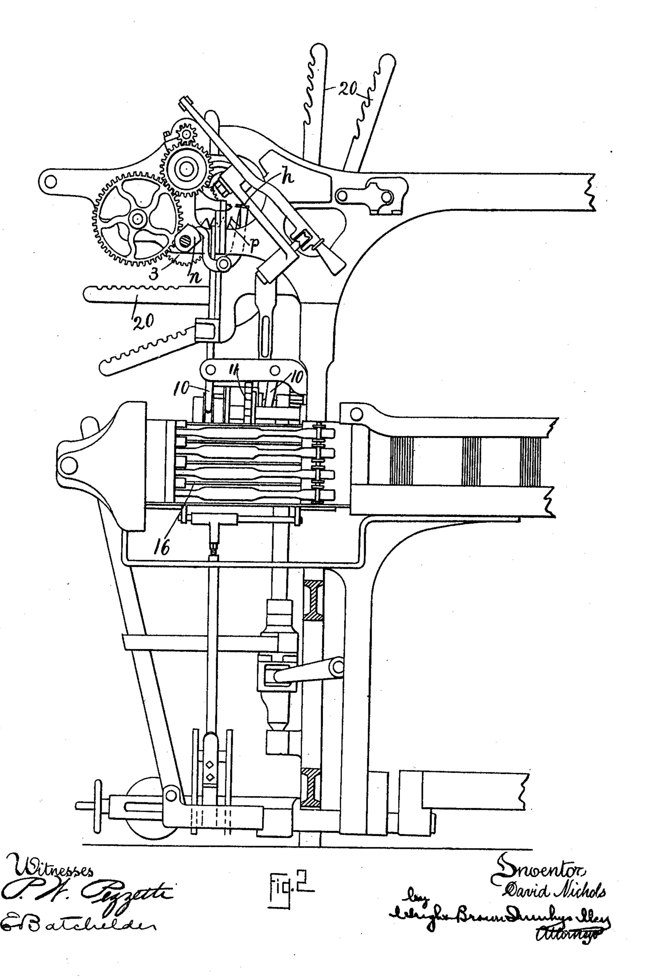
HEALD AND SHUTTLE BOX OPERATING MECHANISM OF LOOMS.
