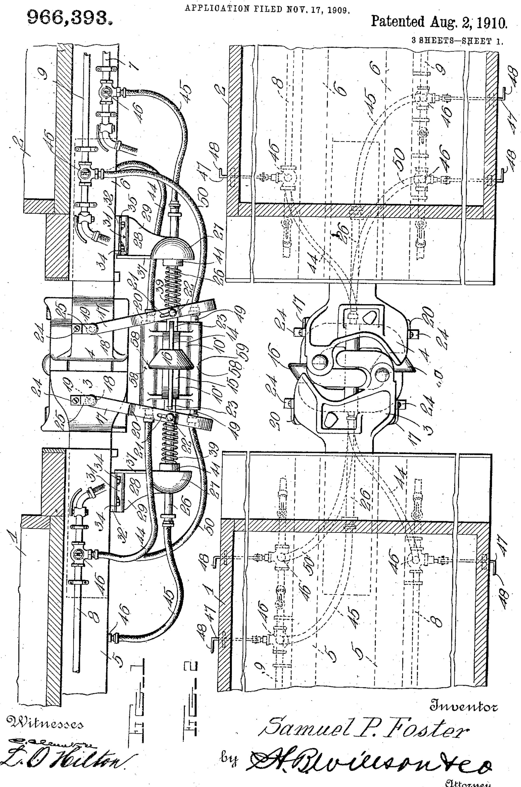
S. P. FOSTER. TRAIN PIPE COUPLING. APPLICATION FILED NOV. 17, 1909.
