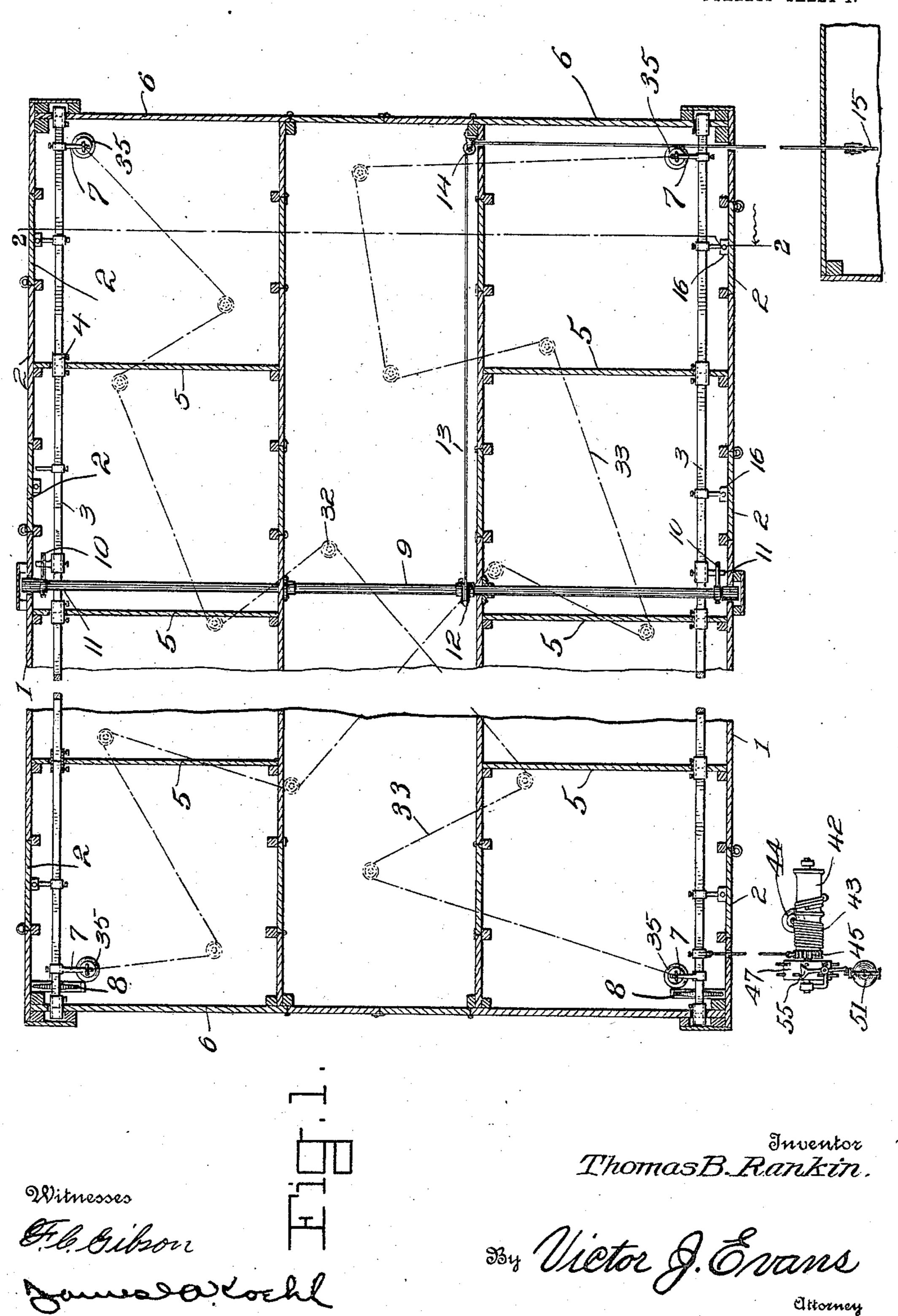
T. B. RANKIN. DOOR RELEASING MECHANISM. APPLICATION FILED DEG. 28, 1909.
