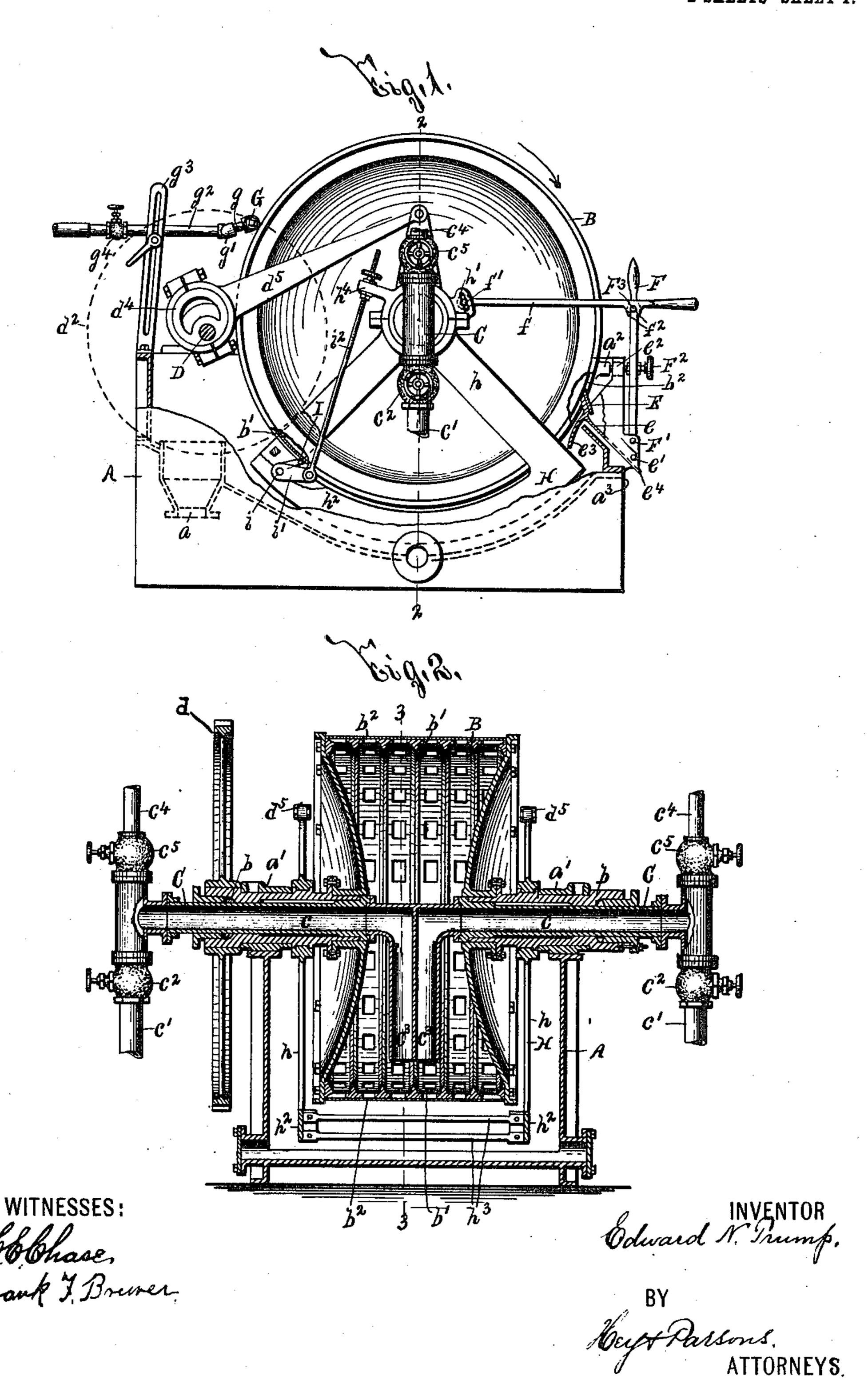
E. N. TRUMP. FILTERING AND DRYING APPARATUS. APPLICATION FILED FEB. 17, 1896.
