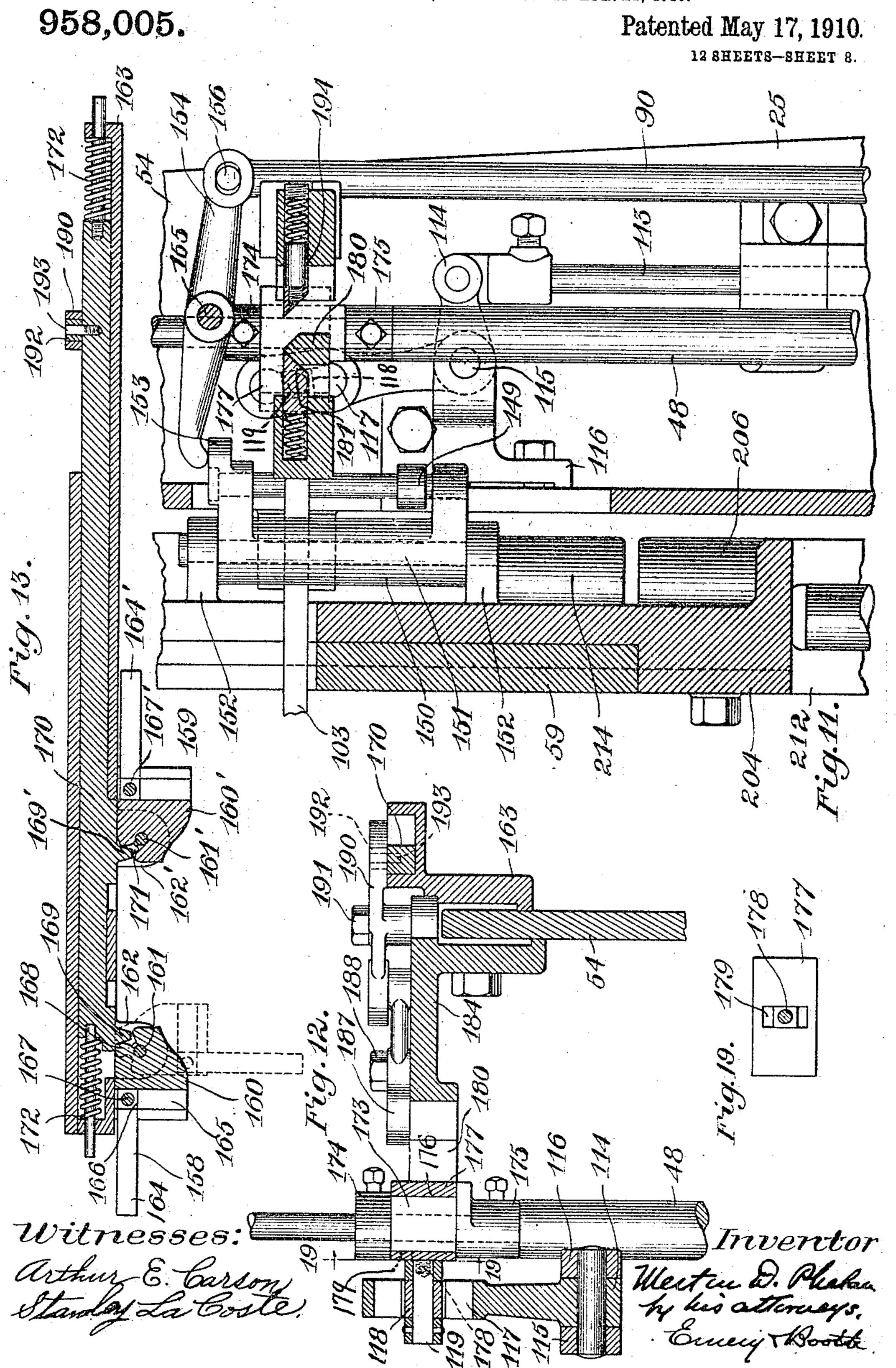
M. D. PHELAN. MACHINE FOR BREASTING THE HEELS OF BOOTS AND SHOES. APPLICATION FILED SEPT. 4, 1906. RENEWED APR. 12, 1910.
