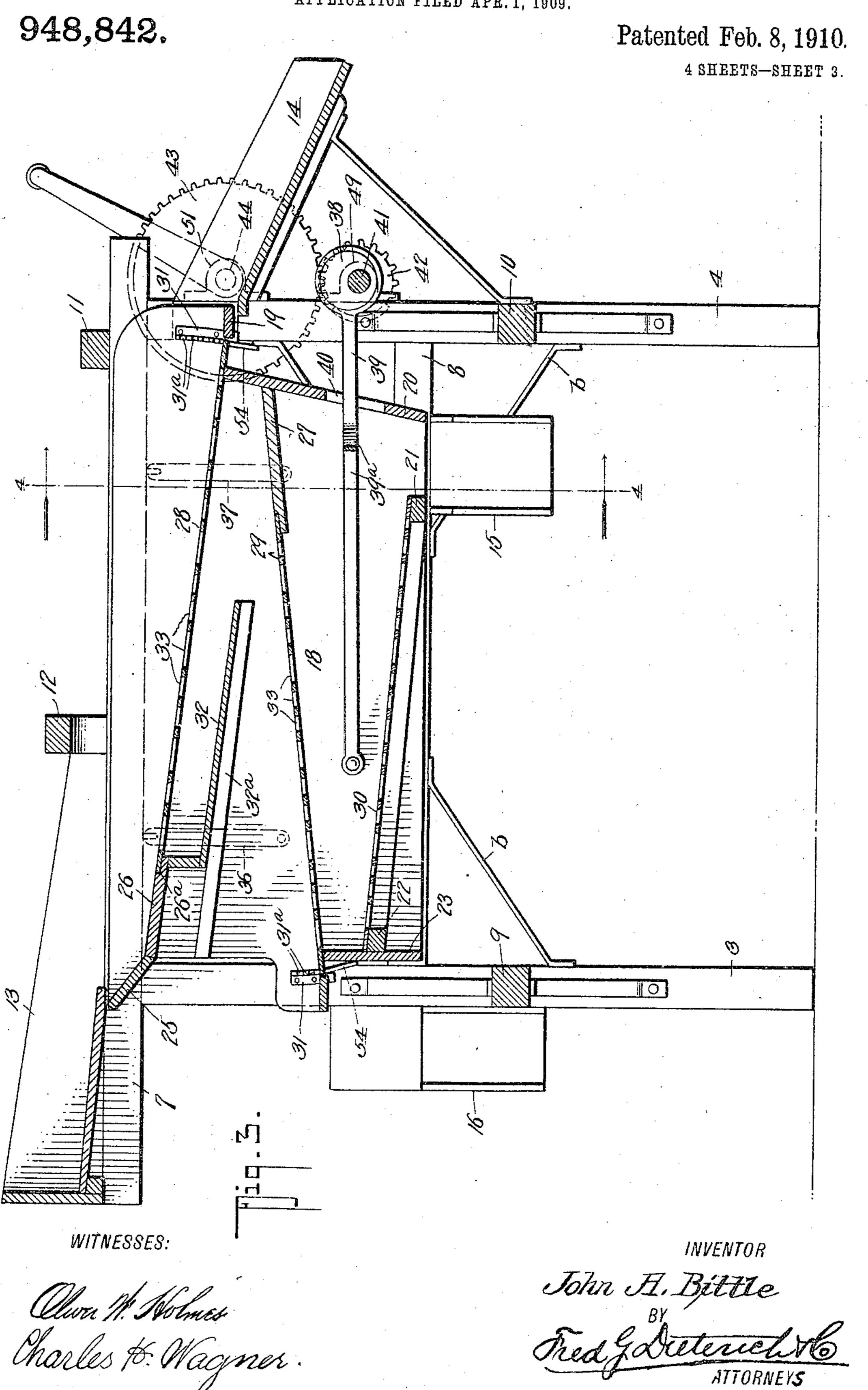
J. A. BITTLE. POTATO CLEANING AND ASSORTING MACHINE. APPLICATION FILED APR. 1, 1909.
