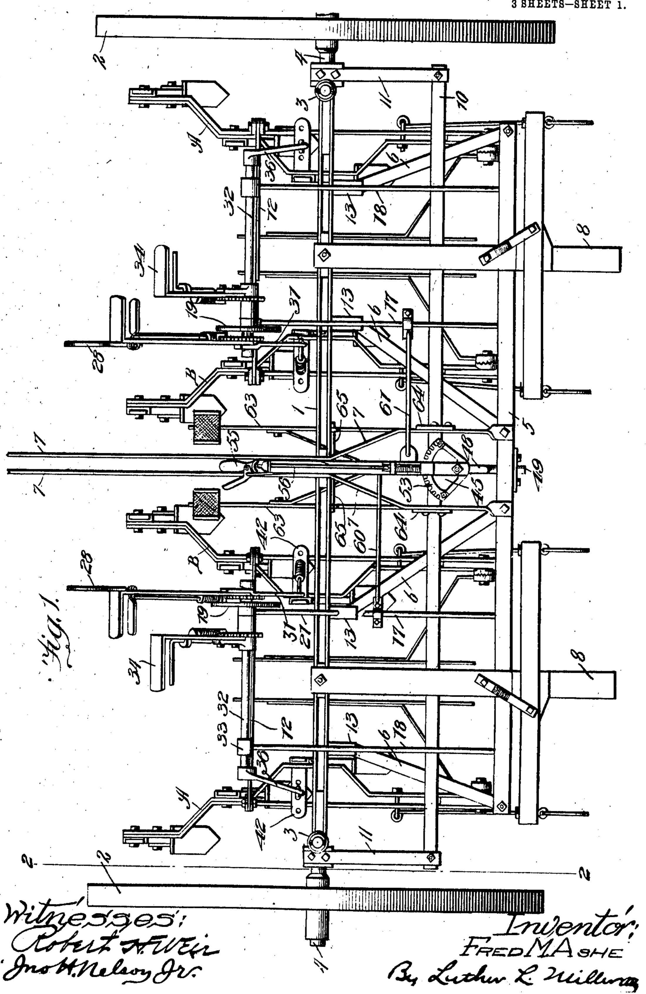
F. M. ASHE. LEVER MECHANISM FOR CULTIVATORS. APPLICATION FILED OCT. 17, 1907.
