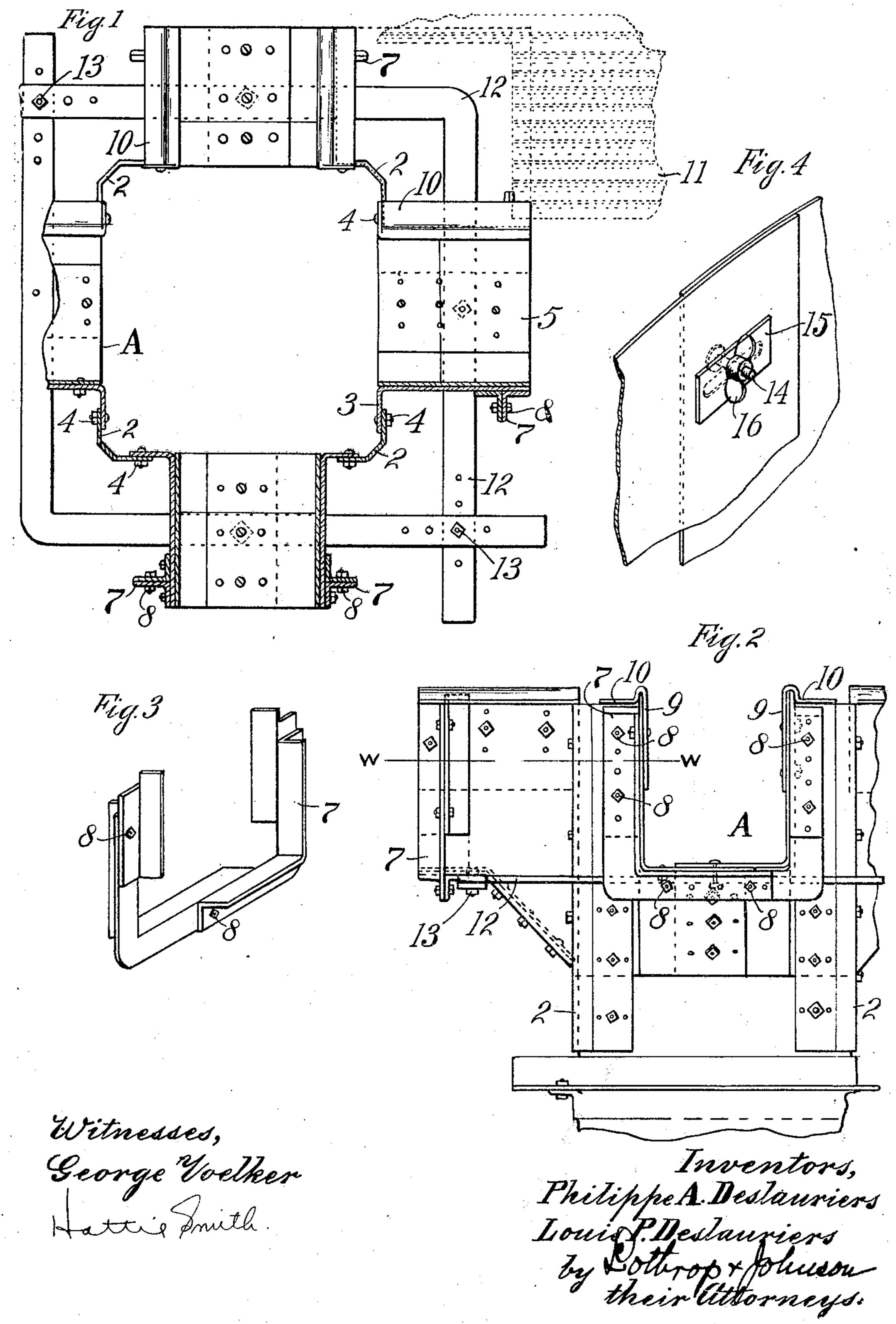
MEANS FOR FORMING CONCRETE CEILINGS AND SUPPORTING COLUMNS. APPLICATION FILED JUNE 29, 1907.
