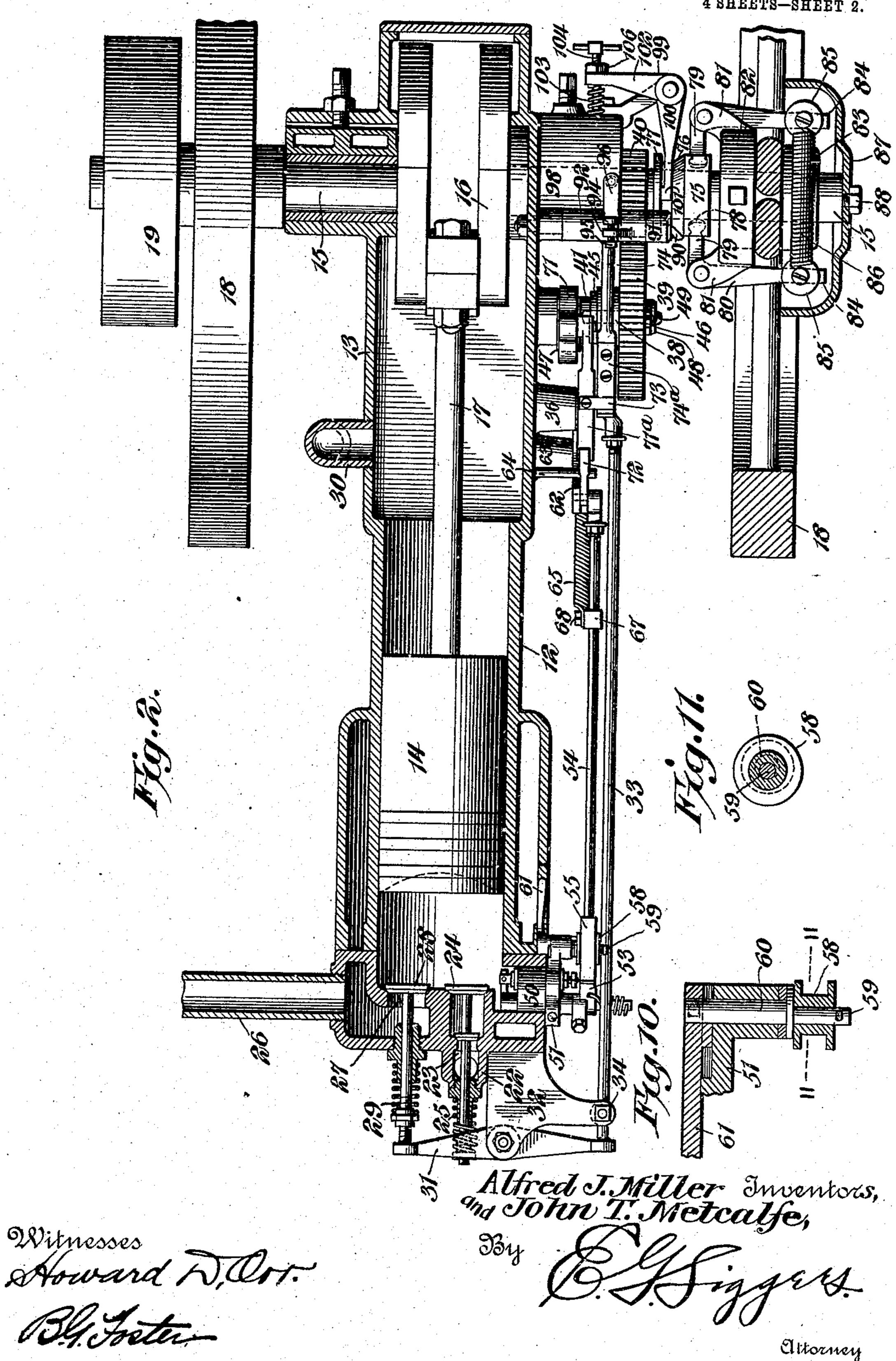
SPEED CONTROLLING MECHANISM FOR EXPLOSIVE ENGINES.
