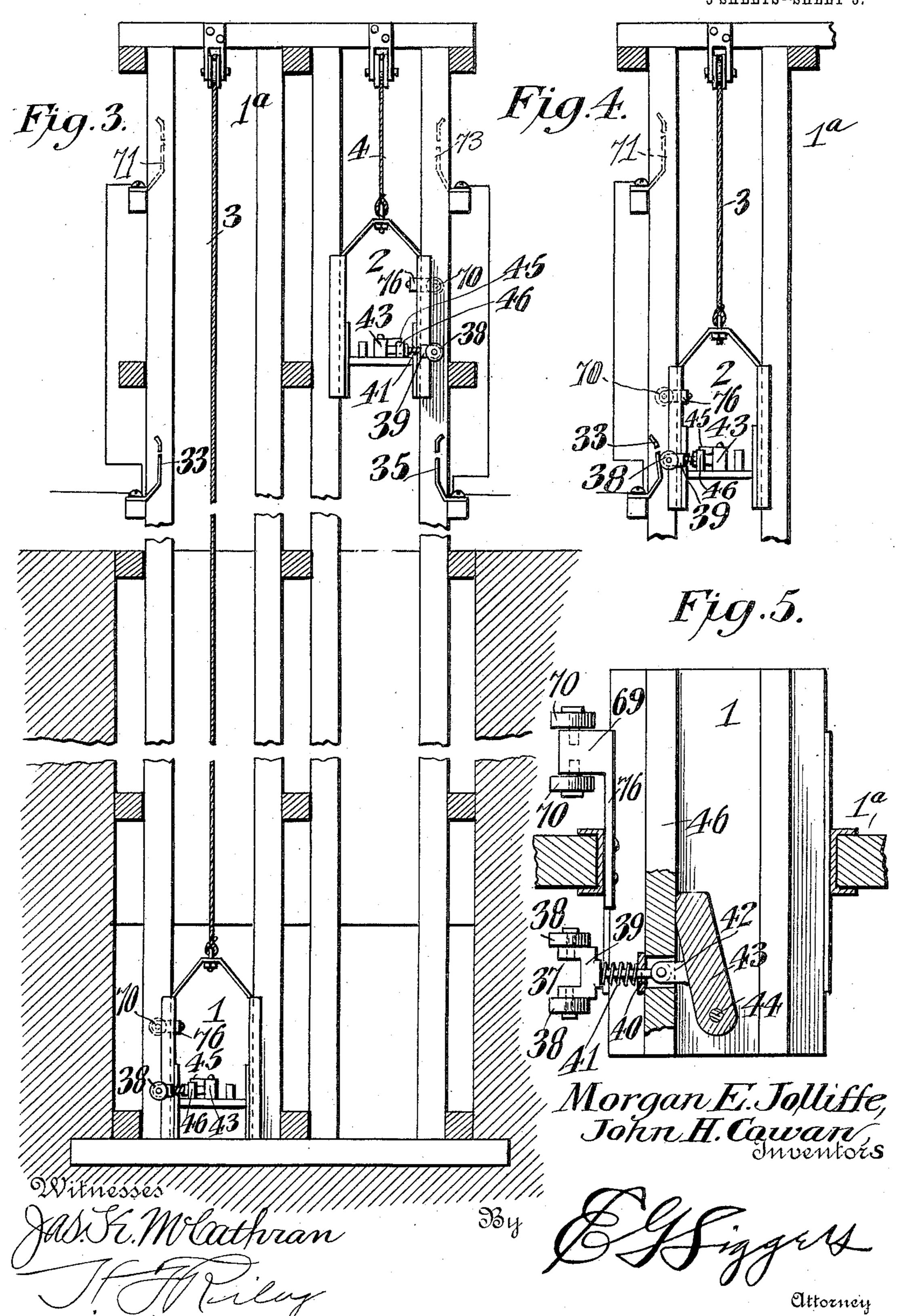
SAFETY ATTACHMENT FOR MINE ELEVATORS.
