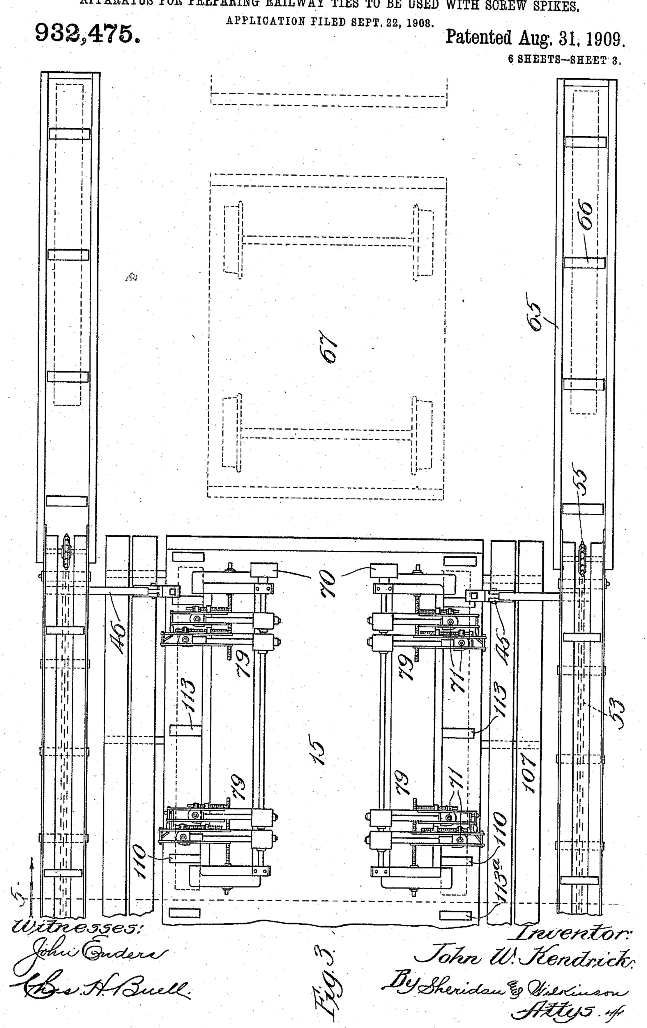
APPARATUS FOR PREPARING RAILWAY TIES TO BE USED WITH SCREW SPIKES.
