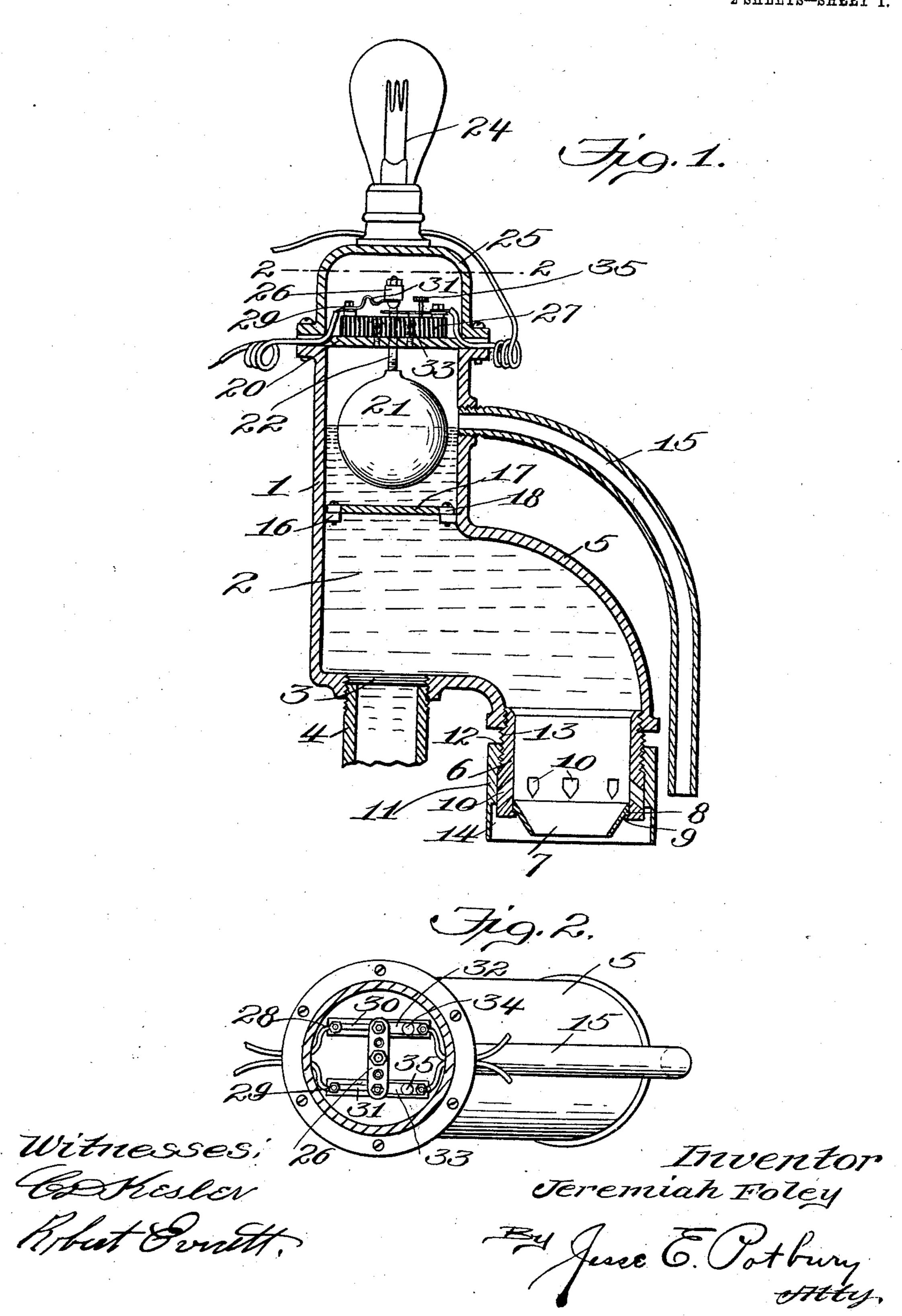
J. FOLEY. LIQUID INDICATOR AND LEAK DETECTOR. APPLICATION FILED NOV. 4, 1908.
