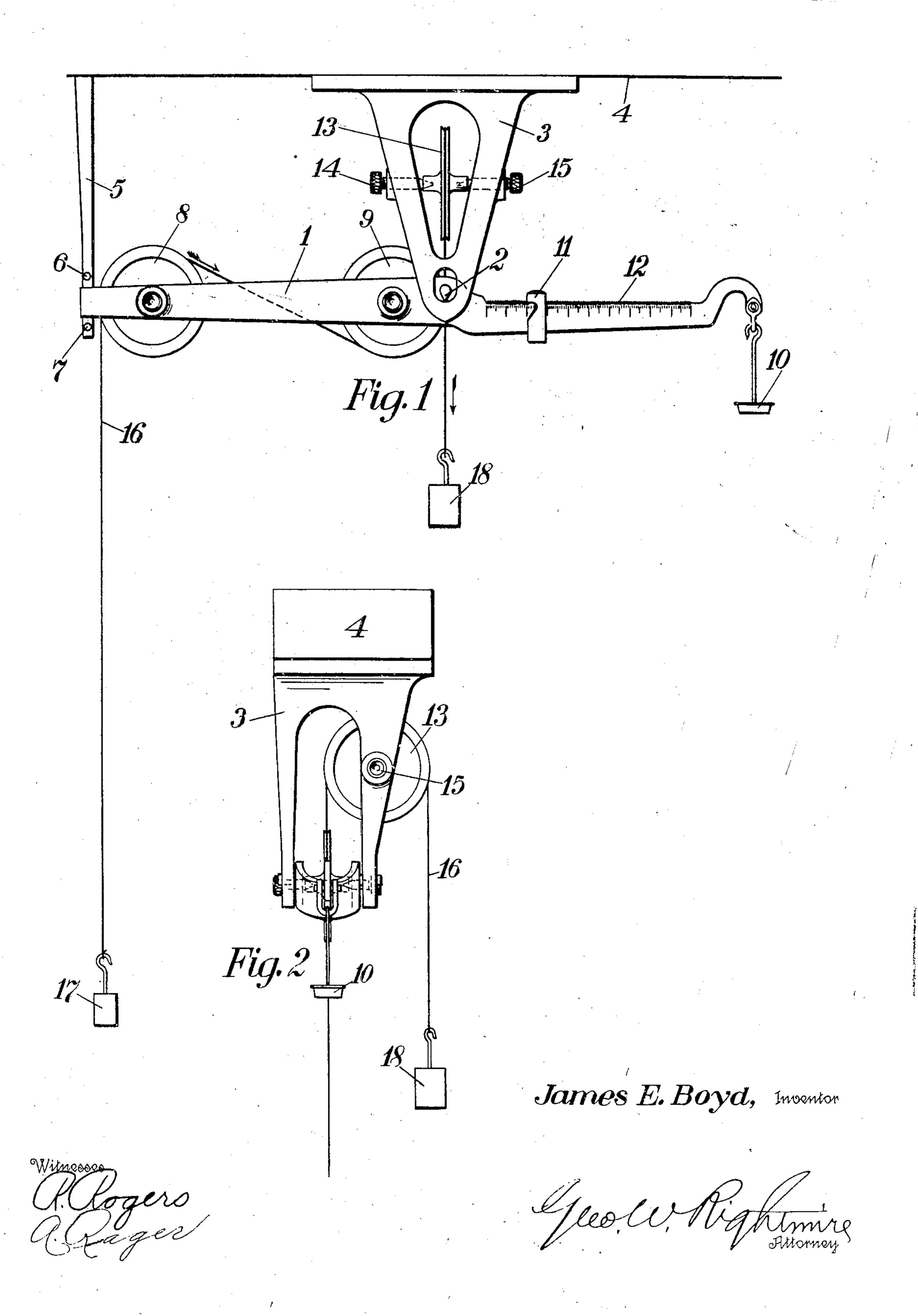
J. E. BOYD. APPARATUS FOR MEASURING ACCELERATION. APPLICATION FILED MAR. 9, 1908.
