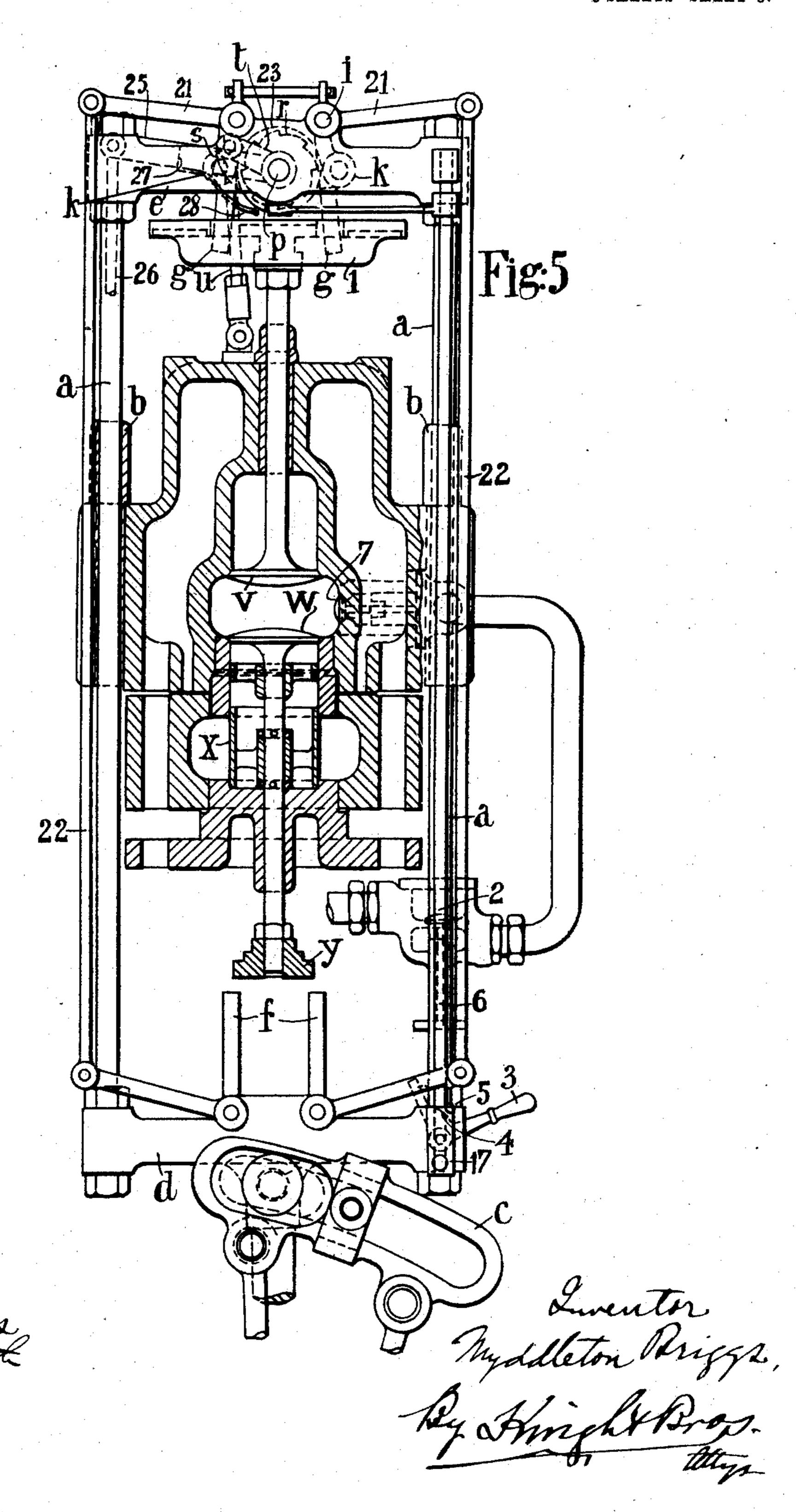
VALVE GEAR AND IGNITION APPARATUS FOR INTERNAL COMBUSTION ENGINES,
