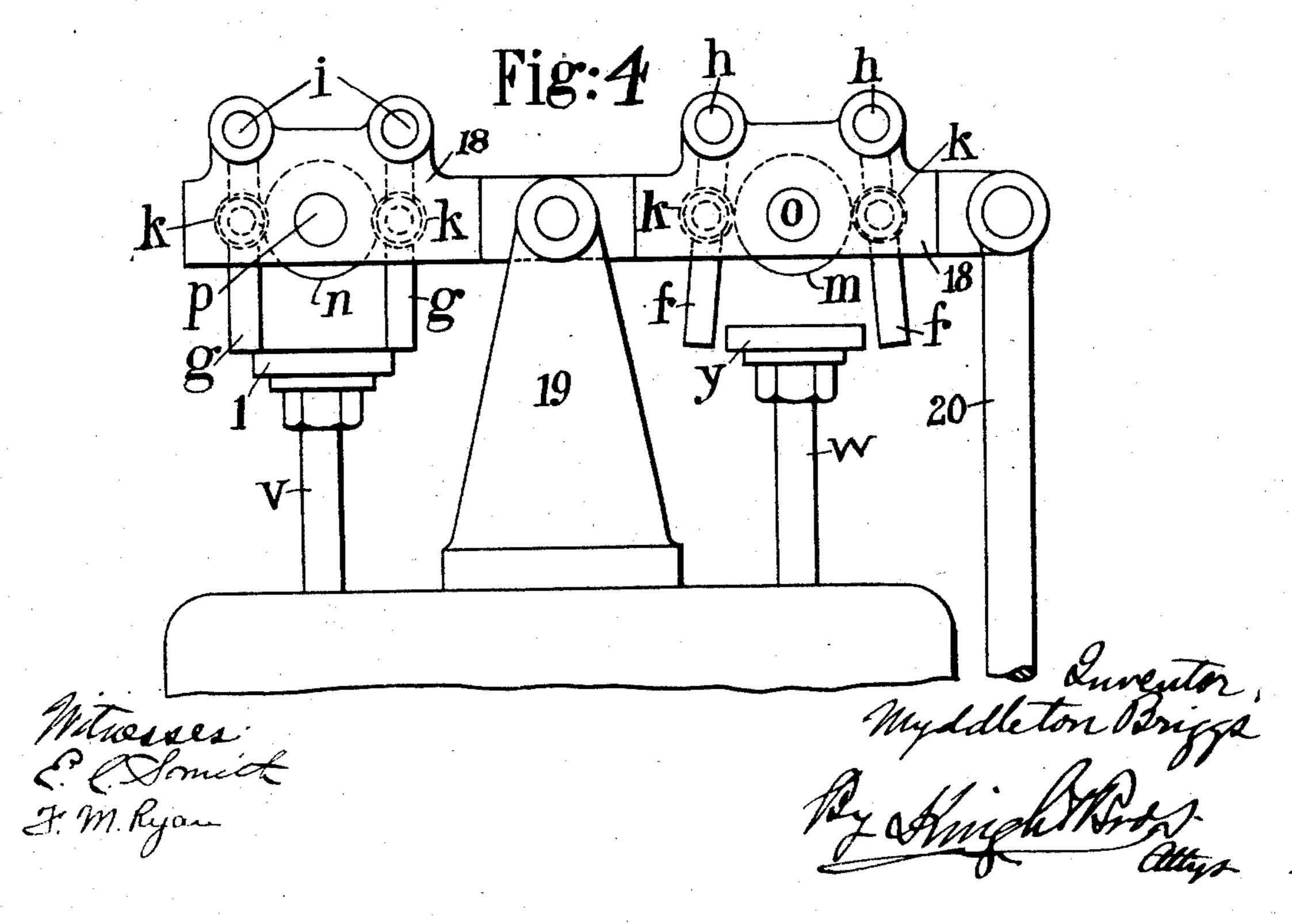
VALVE GEAR AND IGNITION APPARATUS FOR INTERNAL COMBUSTION ENGINES.
