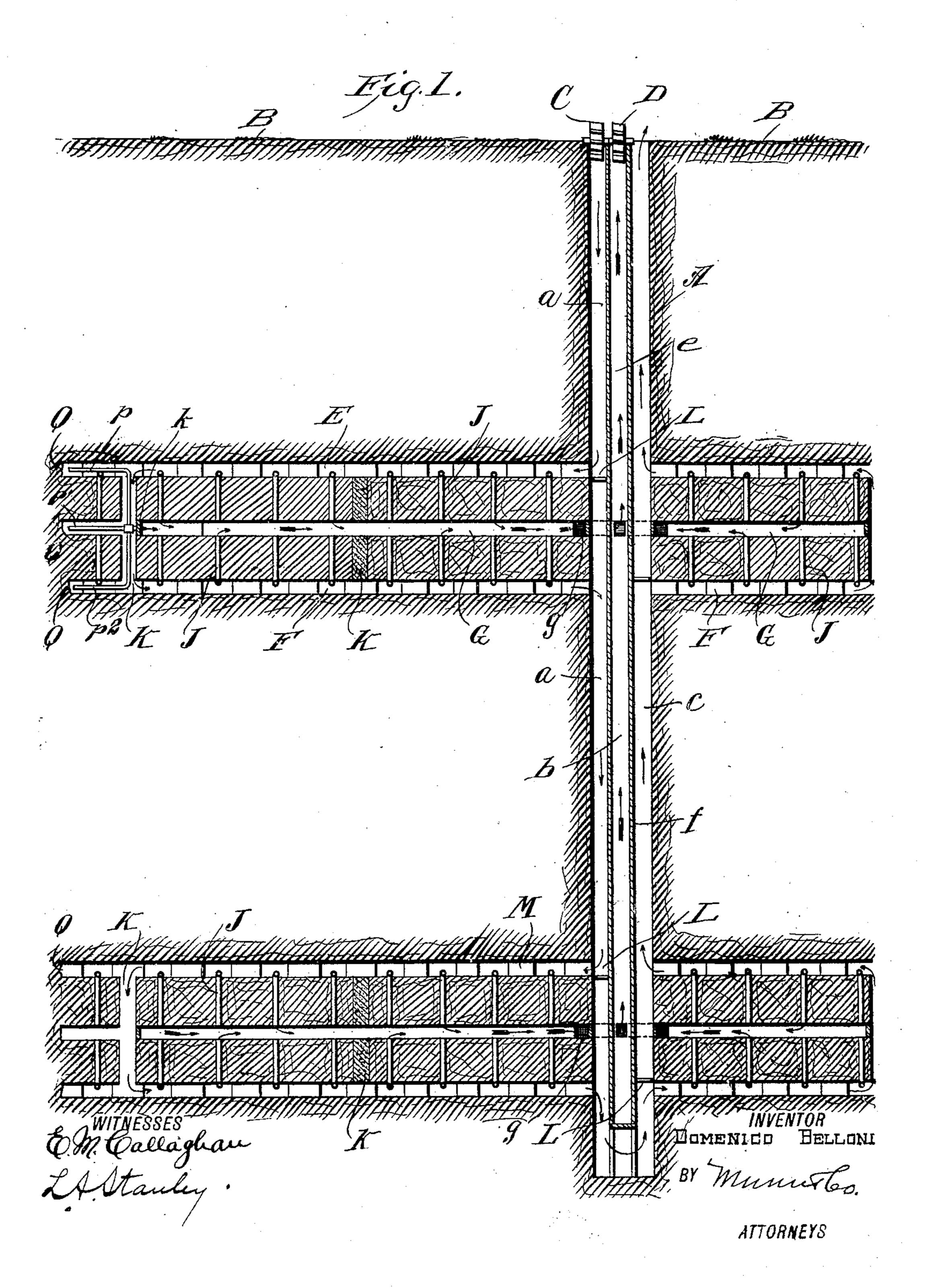
D. BELLONI. SYSTEM OF MINE VENTILATION.
