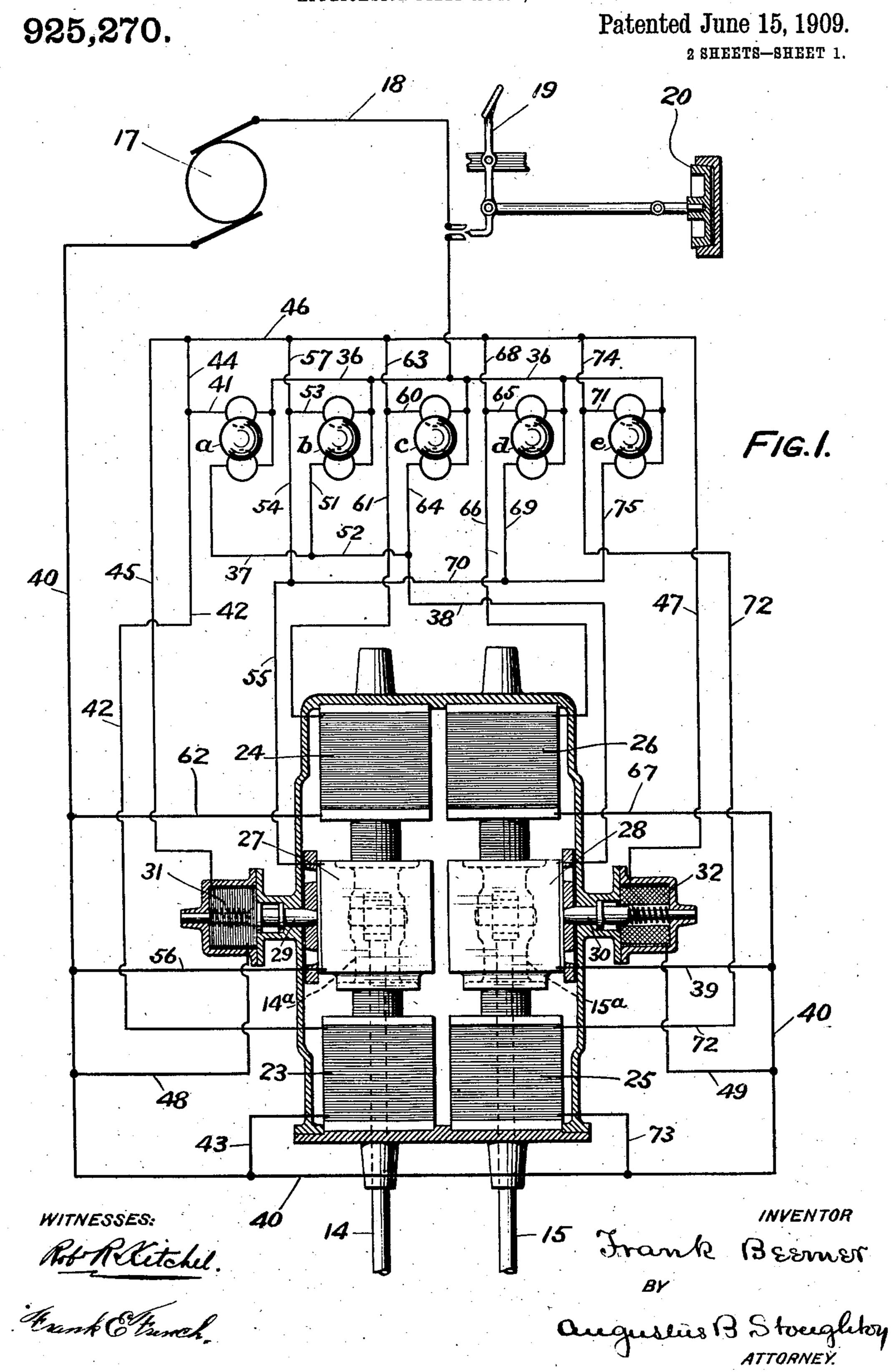
F. BEEMER. ELECTRIC GEAR CHANGING MECHANISM FOR AUTOMOBILES.
