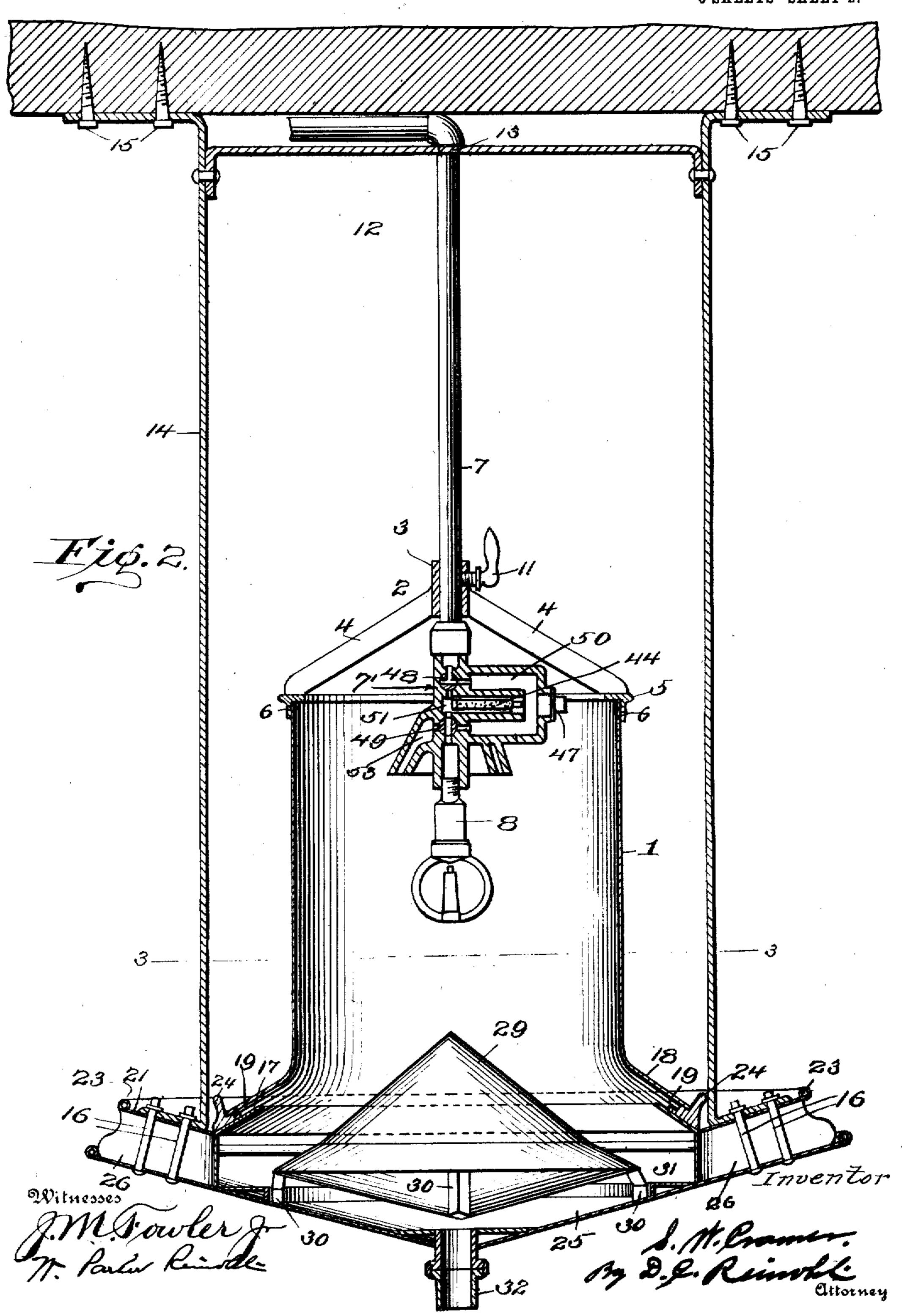
S. W. CRAMER. HUMIDIFIER AND AIR MOISTENING APPARATUS. APPLICATION FILED NOV. 29, 1907.
