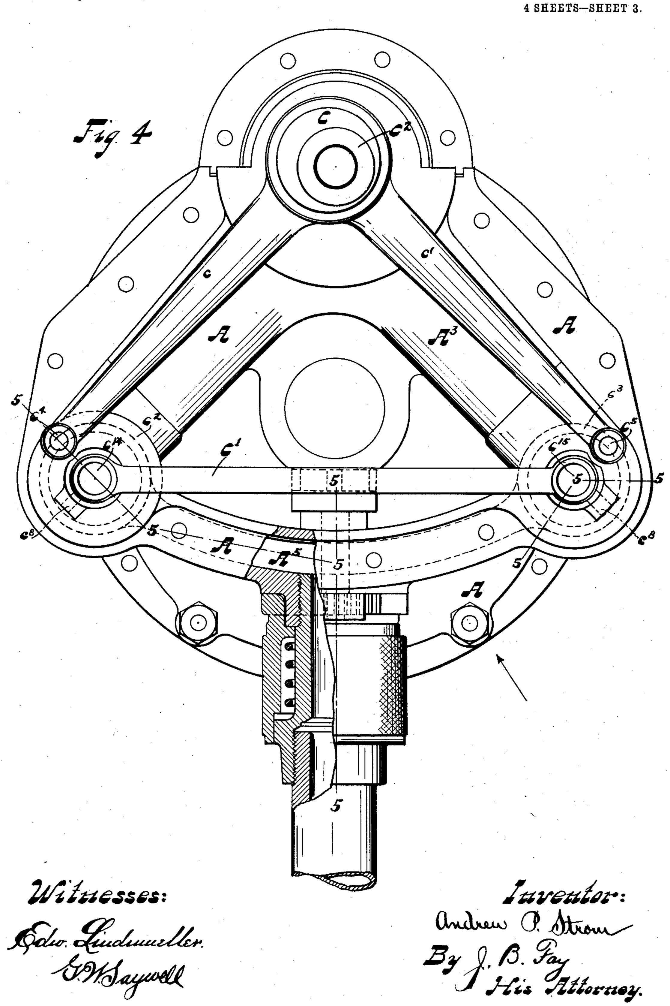
A. P. STROM. PORTABLE PNEUMATIC DRILL. APPLICATION FILED APR. 5, 1906.
