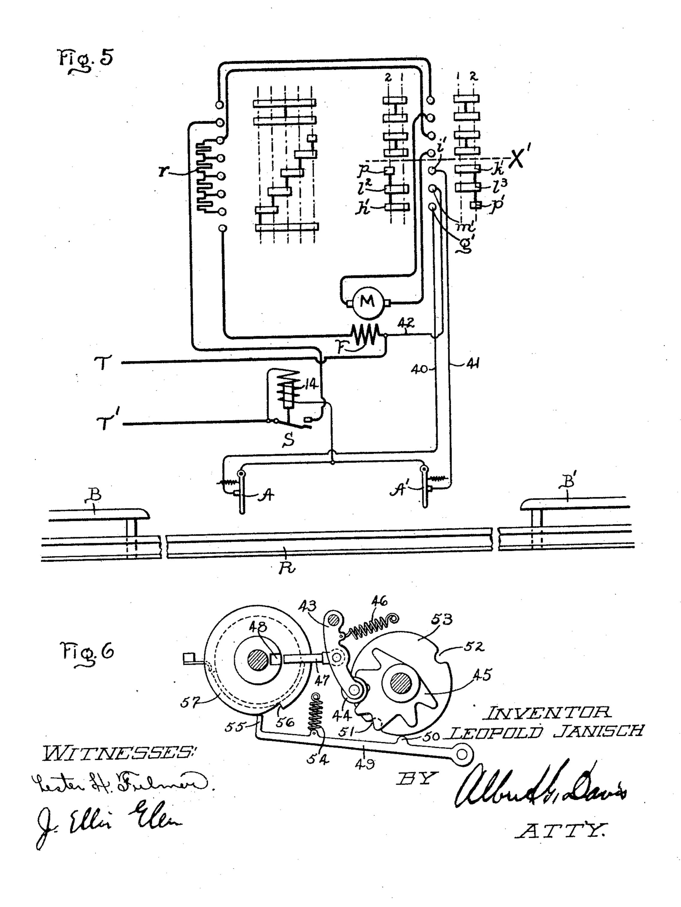
CONTROL SYSTEM FOR MOTOR DRIVEN RECIPROCATING DEVICES.
