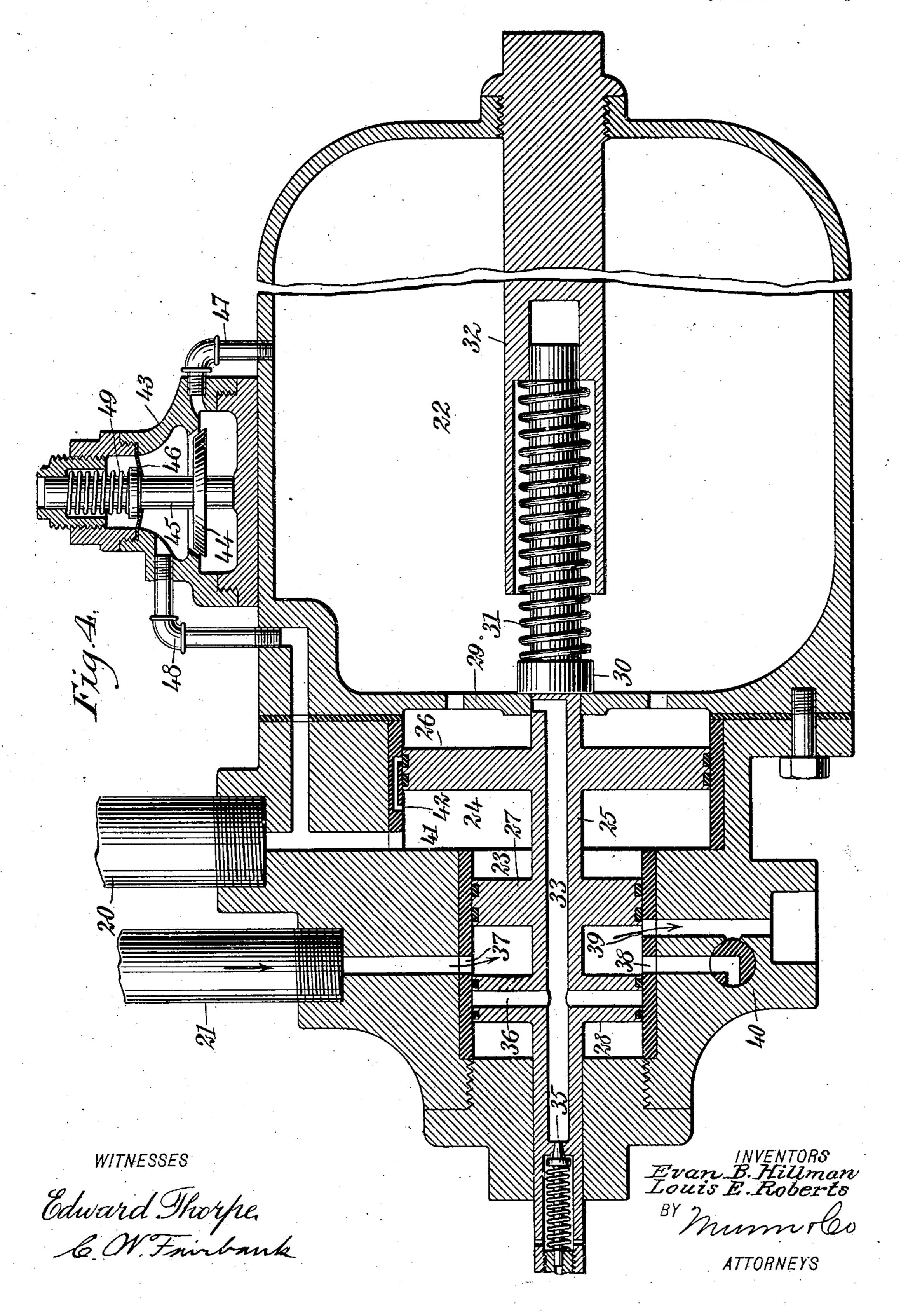
E. B. HILLMAN & L. E. ROBERTS. AUTOMATIC PRESSURE RETAINING AND GRADUATING RELEASE DEVICE FOR AIR BRAKES.
