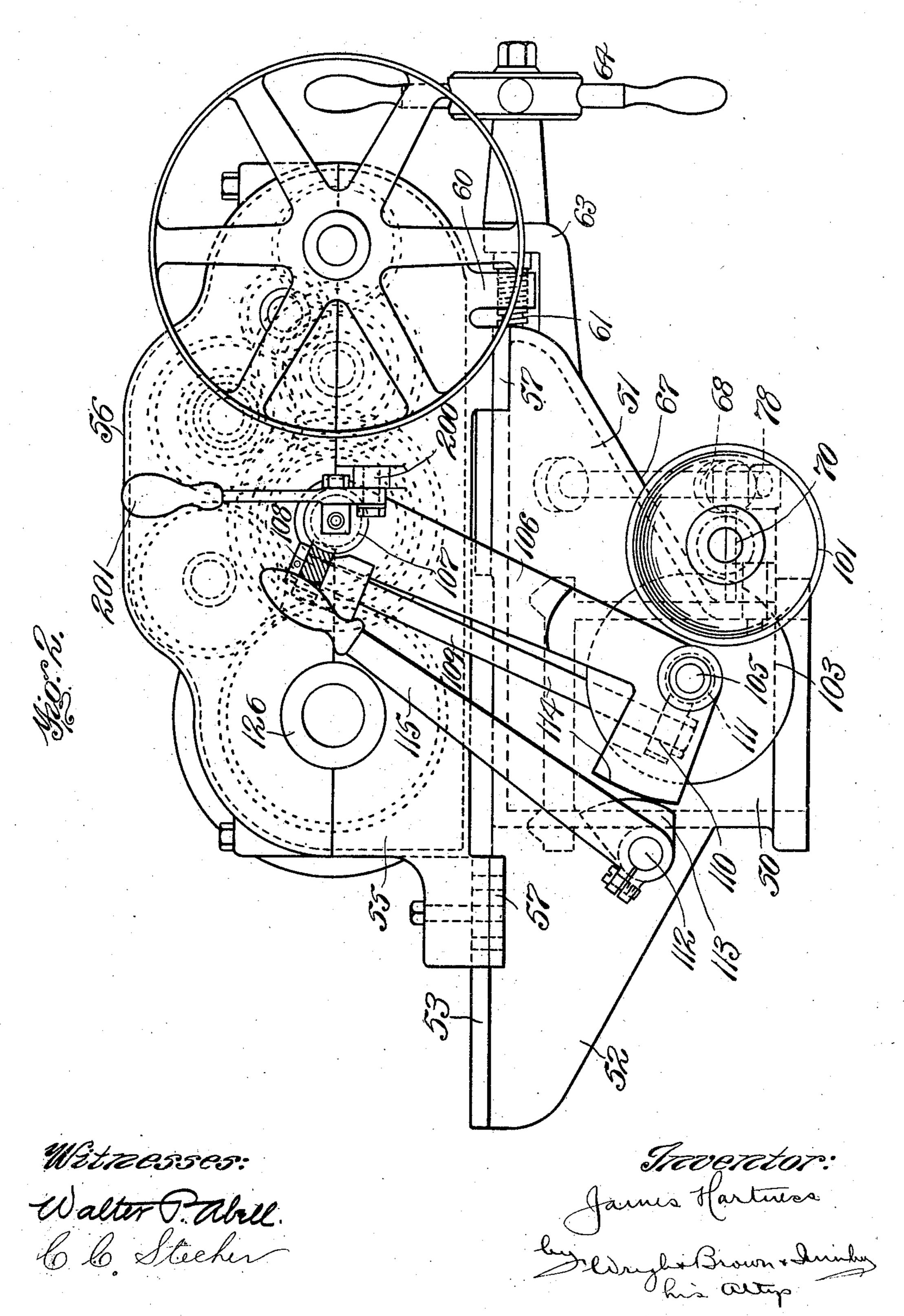
POWER TRANSMITTING MECHANISM FOR METAL WORKING MACHINES
