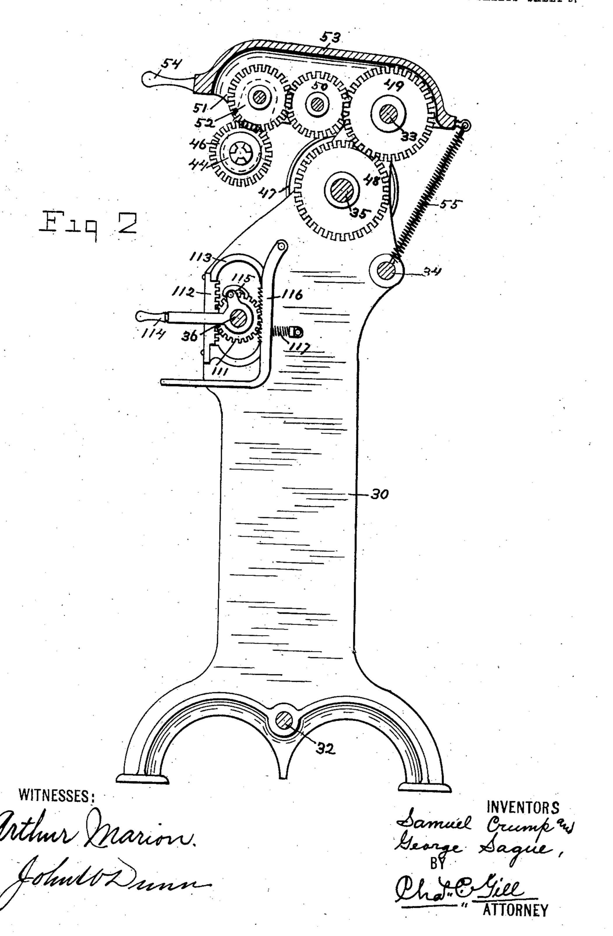
MACHINE FOR CLEANING OR TREATING PRINTERS' ROLLERS.
