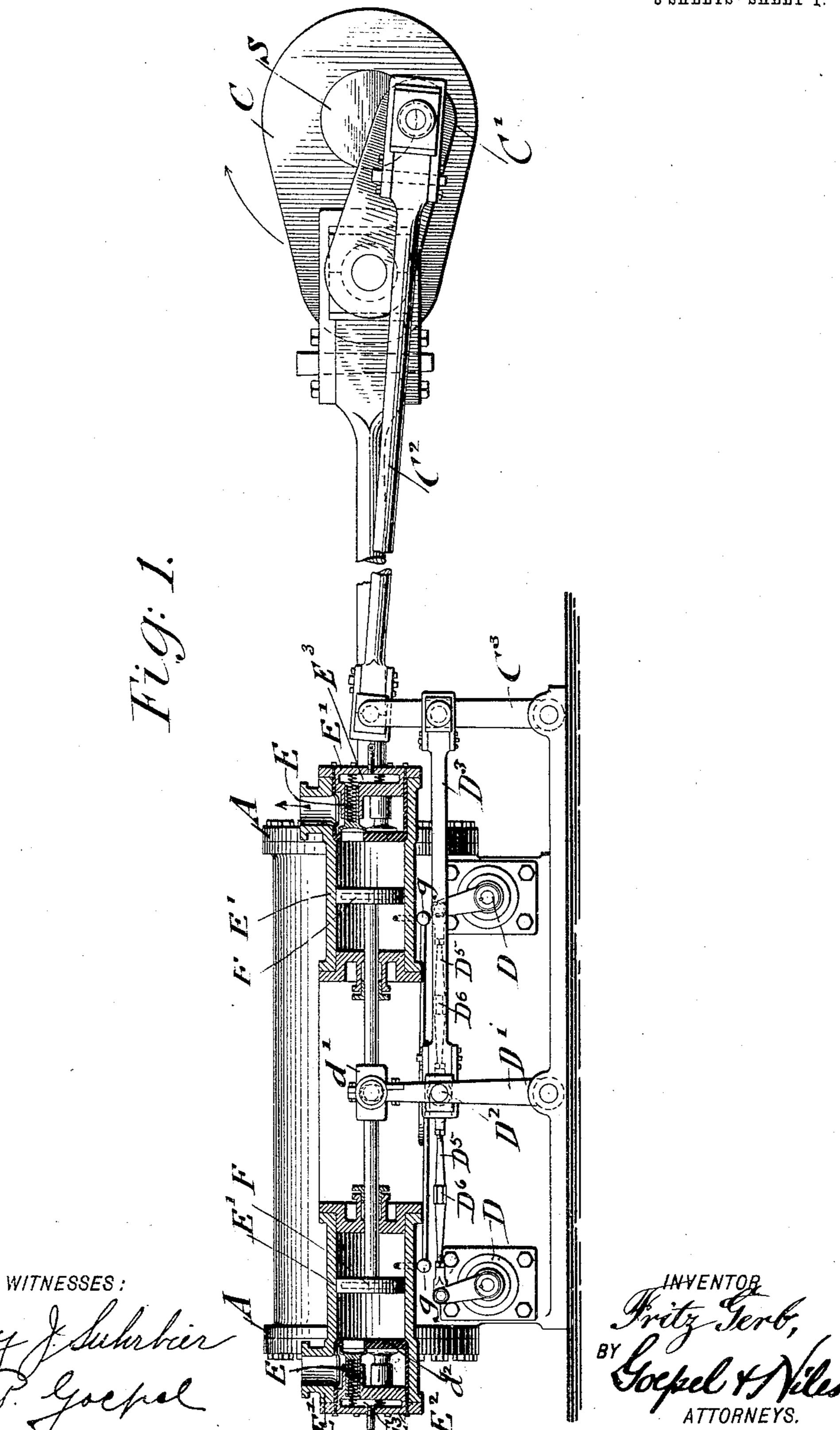
F. GERB. VALVE MOTION FOR AIR COMPRESSORS. APPLICATION FILED SEPT. 16, 1902.
