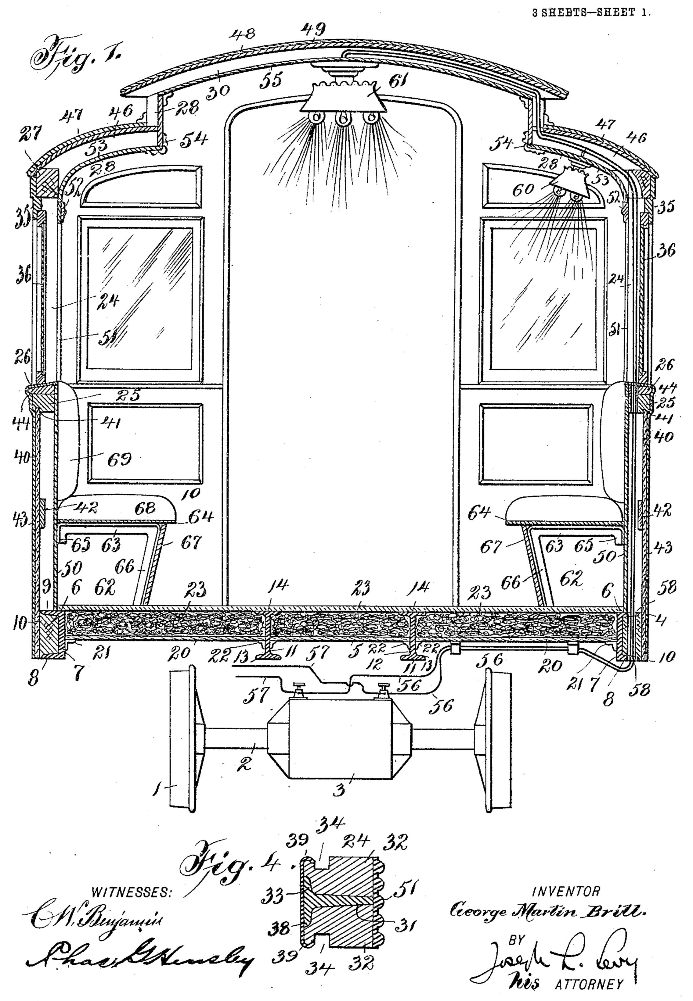
G. M. BRILL. CONSTRUCTION OF RAILWAY CARS. APPLICATION FILED NOV. 24, 1903.
