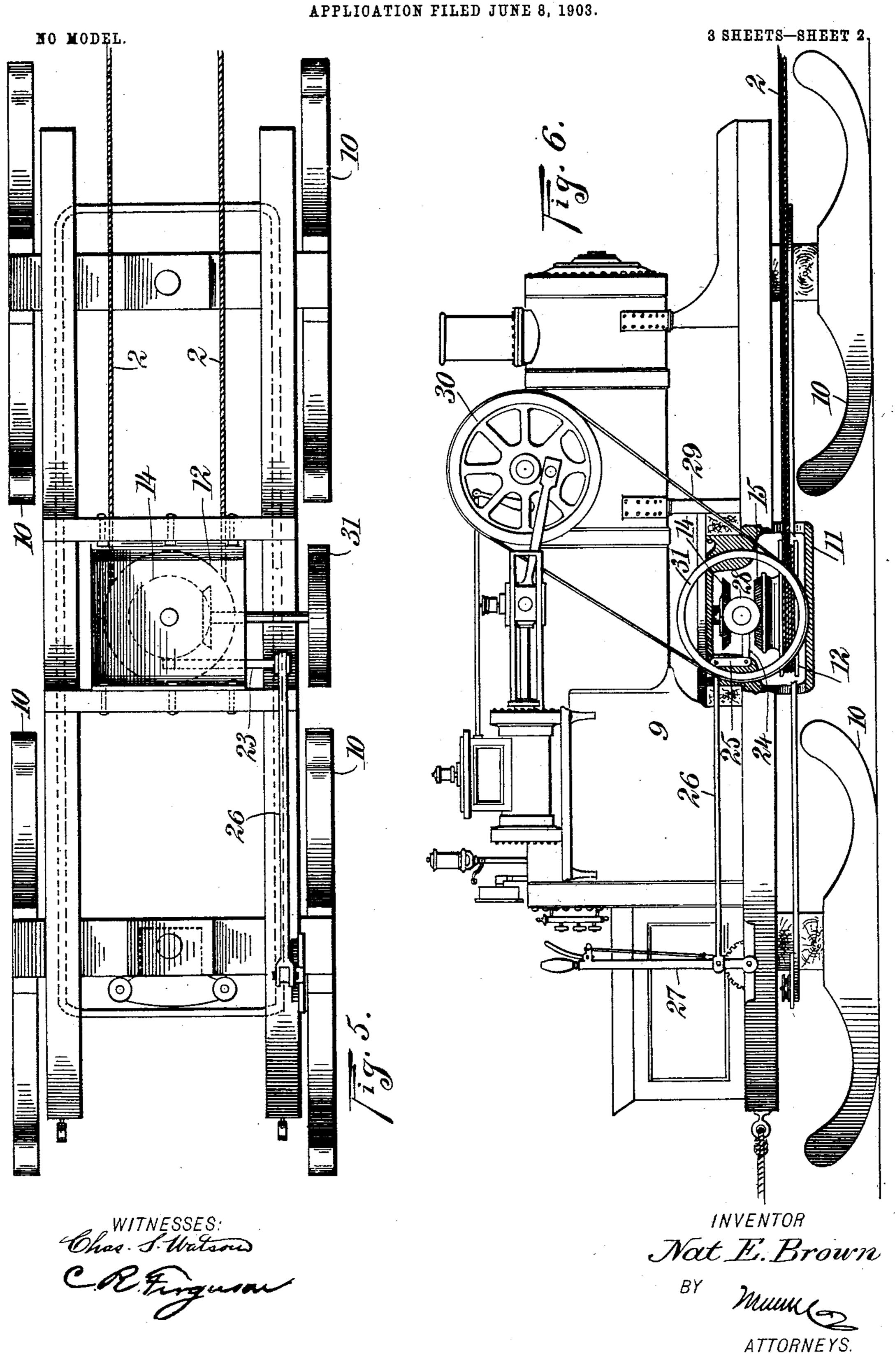
DRAFT MECHANISM FOR TRACTION SLEDS.
