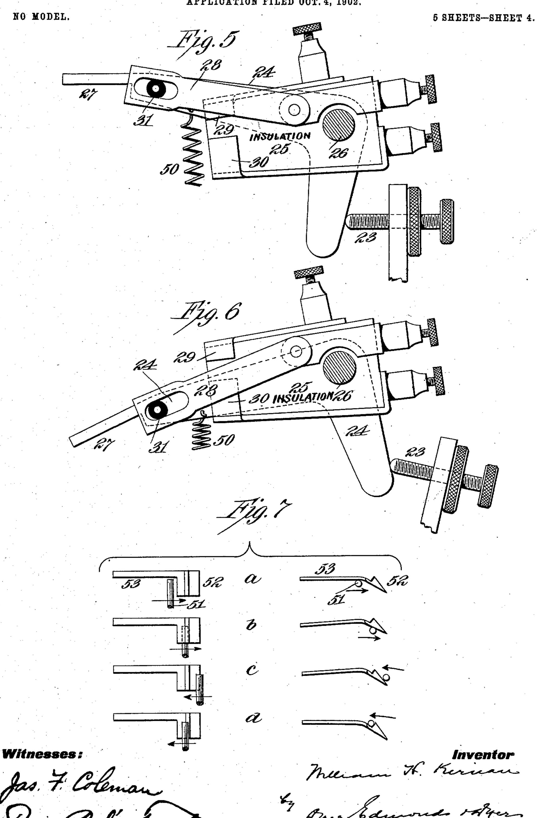
AUTOMATIC NON-INTERFERING REPEATER FOR FIRE ALARM CIRCUITS.
