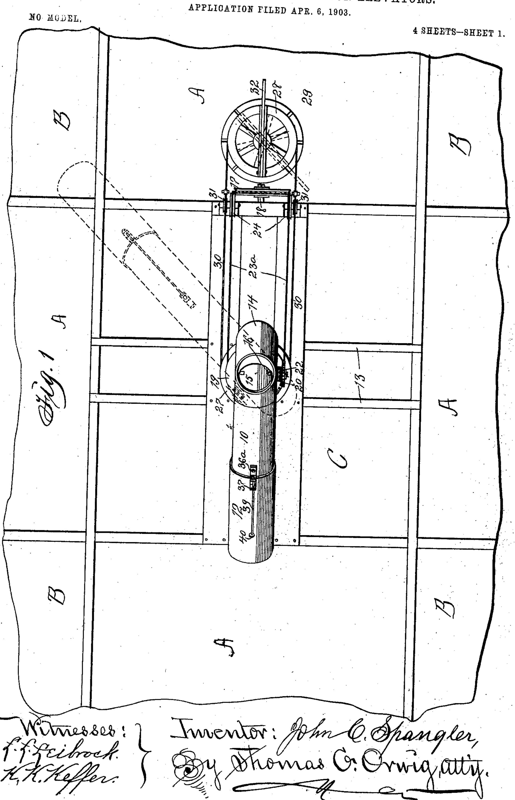
J. C. SPANGLER. ROTATABLE GRAIN DISTRIBUTER FOR ELEVATORS.
